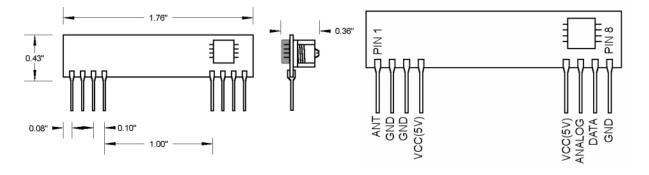
Figure 1. Mechanical Drawing
