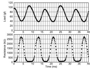
response data are shown in the graph on the left. The data in the graph on the right were taken after 9,000,000 cycles were applied to the sensor material. Each cycle consisted of 100g applied for one second and no load for 1 second.
