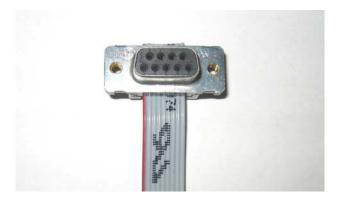
2) Next, the opposite end of the ribbon cable needs to have some of its wires shortened. The serial connection only needs 3 of the 9 (transmit, receive, and ground) signals. Cut and strip the opposite end of the cable so that it looks like the following photo:
