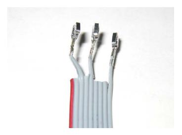
4) Insert the three metal crimp connectors into the white Molex housing, ensuring that the catch on each connector locks securely in place. NOTE: This step requires that second and fourth wire (from the red strip in the ribbon cable) are crossed over before inserting into the housing, as shown in the following photo:
