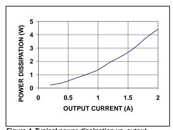
Figure 4. Typical power dissipation vs. output current.
