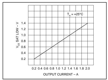
Figure 2. Typical sink saturation voltages vs. load current
