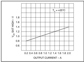
Figure 1. Typical source saturation voltages vs. load current
