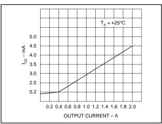
Figure 3. Typical supply current vs. load current.
