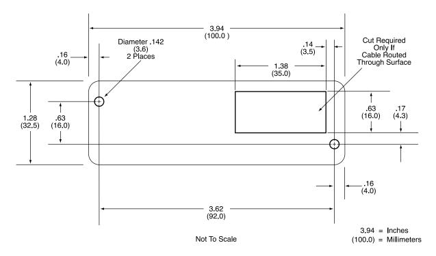
Figure 2-1. Mounting Hole Dimensions for Surface
