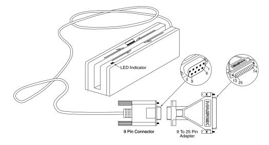
Figure 1-2. Reader Cable and Optional Adapter
