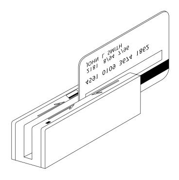
Figure 1-1. Port-Powered Swipe Reader
