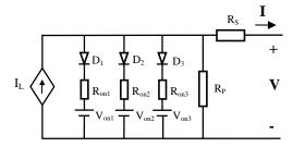
Fig. 5a Proposed PWL Model of PV cell
