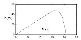
Fig. 7 P-V curve with the proposed model
