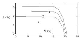
Fig. 8 I-V family curves with proposed model for different irradiation levels
