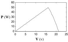
Fig. 11 P-V curve with classical model
