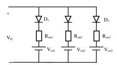
Fig. 4 Proposed PWL Model of PV diode
