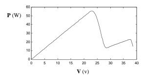
Fig. 12 P-V curve of simulated mismatched PV Panels
