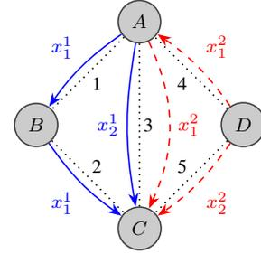
Fig. 1. A sample network with five links (dotted line) and two users. The first user, whose source is  $A$  and destination is  $C$ , has rate  $x_1^1$  and  $x_2^1$  on its two paths (solid line). The second user, whose source is  $D$  and destination is  $C$ , has rate  $x_1^2$  and  $x_2^2$  on its two paths (dashed line).
