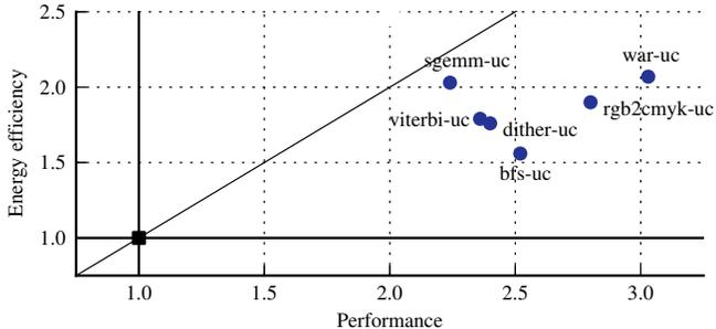
Figure 10. VLSI Energy Efficiency vs. Performance – Compares the in-order GPP augmented with the LPSU normalized to baseline the in-order processor. Diagonal line is the iso-power contour.
