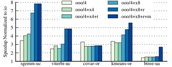
Figure 9. Microarchitectural Design Space Exploration Speedups – Normalized to running baseline kernel on  $io$ .  $ooo/4$  = 4-way out-of-order processor;  $x4/x8$  = LPSU design with 4 and 8 lanes, respectively;  $r$  = additional LLFUs and data memory ports;  $t$  = 2-way multithreading;  $m$  = additional LSQs.
