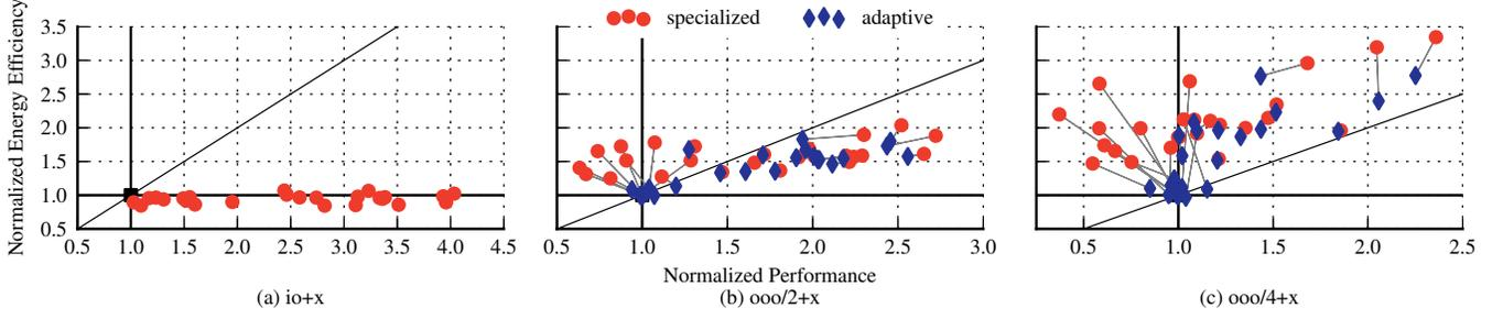
Figure 8. Energy Efficiency vs. Performance – Cycle-level performance and McPAT energy results of specialized and adaptive execution for (a)  $io+x$  normalized to  $io$ , (b)  $ooo/2+x$  normalized to  $ooo/2$ , (c)  $ooo/4+x$  normalized to  $ooo/4$ . Diagonal lines are iso-power contours.
