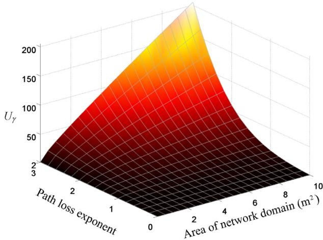
**Fig. 1: Upper bound on  $N_t^Q$  as a function of the area of the network domain and the path loss exponent**
