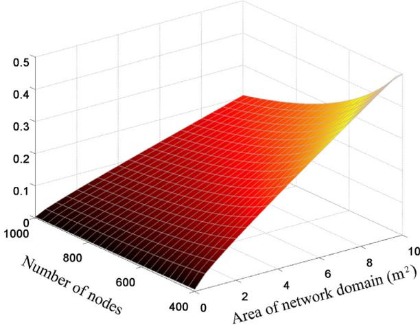
**Fig. 3: Upper bound on the normalized  $\lambda_e$  and  $\lambda_m$  as a function of the area of the network domain and the number of nodes**
