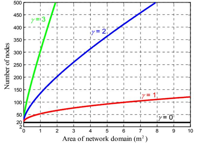
**Fig. 4: Curves formed by the  $(A,N)$  pairs for which  $A_U=0.1$ . For the  $(A,N)$  pairs above the curves, any normalized throughput greater than or equal to 0.1 is not achievable**
