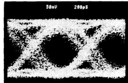
Fig. 17. Eye diagram for the MM-MM-SM experiment.
