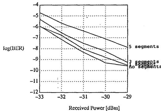
Fig. 20. The effect of splices on the BER performance.
