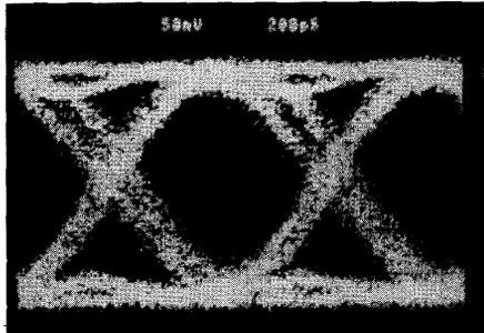
Fig. 19. Eye diagram for the SM-SM-SM experiment.
