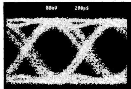
Fig. 18. Eye diagram for the SM-MM-SM experiment.
