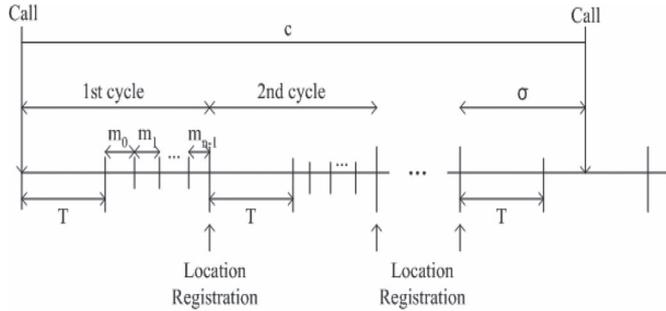
Fig. 2. Time diagram of the hybrid location-update scheme.
