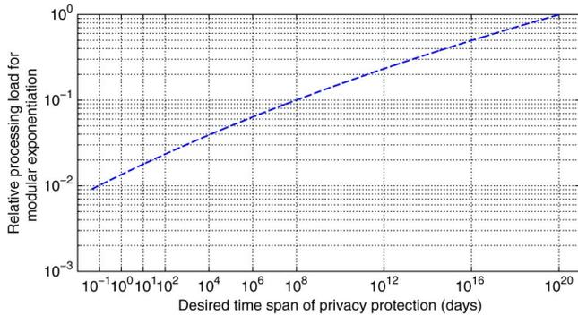
Fig. 4. Relative processing load for modular exponentiation operation versus the desired time span of privacy protection in days.
