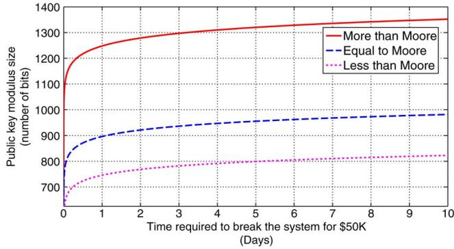
Fig. 3. Public key modulus size versus the number of days required to break the crypto system for \$50 K in the year 2025 under different technology growth rates.
