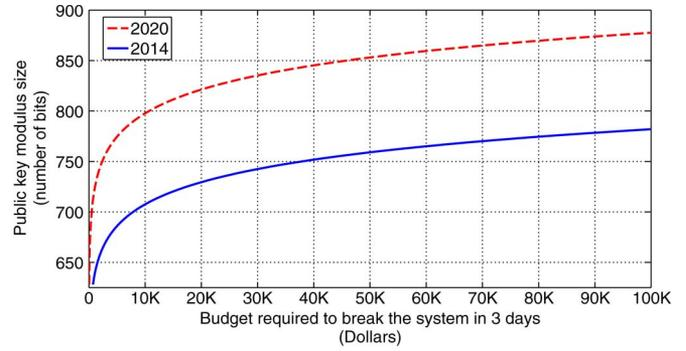
Fig. 2. Public key modulus size versus the Dollar budget required to break the crypto system in 3 days in the year 2014 and year 2020.
