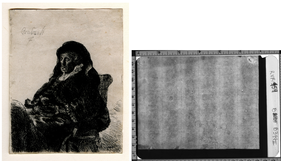
Figure 9: Pupil of Rembrandt, The Artist's Mother in Widow's Dress and Black Gloves (B344) is shown on the left. A beta-radiograph of the area near the watermark is shown on the right. Thanks are extended to Reba Snyder for providing the beta-radiograph of B344. (Etching Photo Credit: The Morgan Library & Museum, New York. RvR 459. Photography by Graham S. Haber, 2014.)
