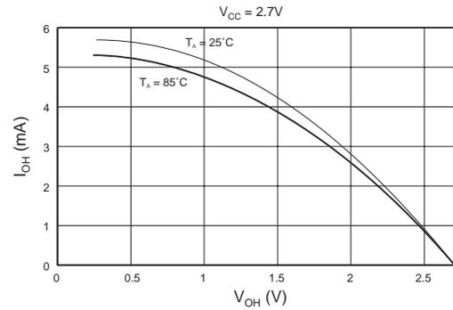
I/O PIN SINK CURRENT vs. OUTPUT VOLTAGE
