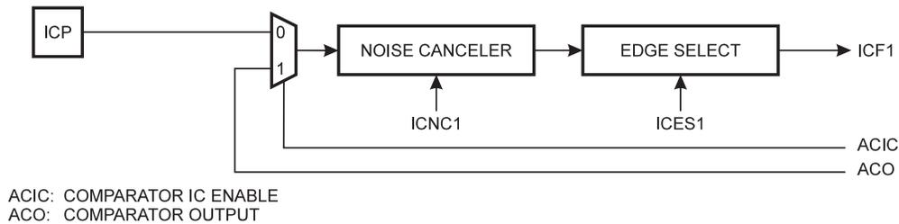
If the noise canceler function is enabled, the actual trigger condition for the capture event is monitored over 4 samples
