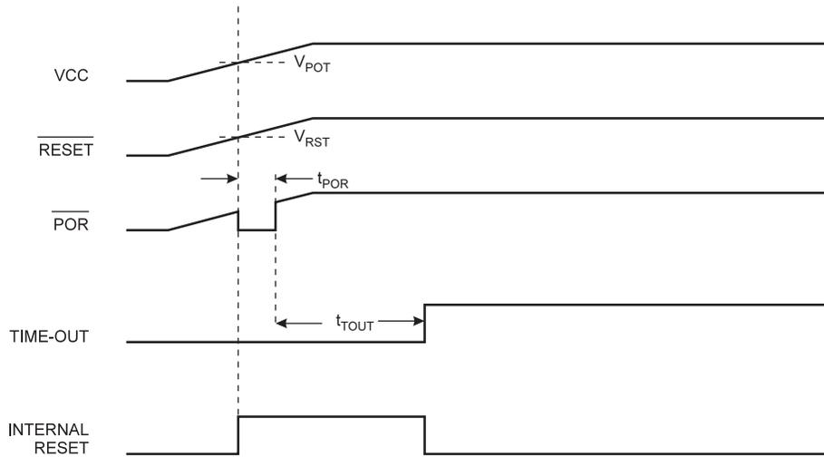
Figure 28. MCU Start-Up,  $\overline{\text{RESET}}$  Controlled Externally
