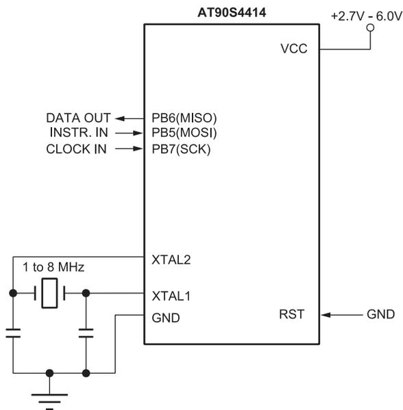
When writing serial data to the AT90S4414, data is clocked on the rising edge of CLK.
