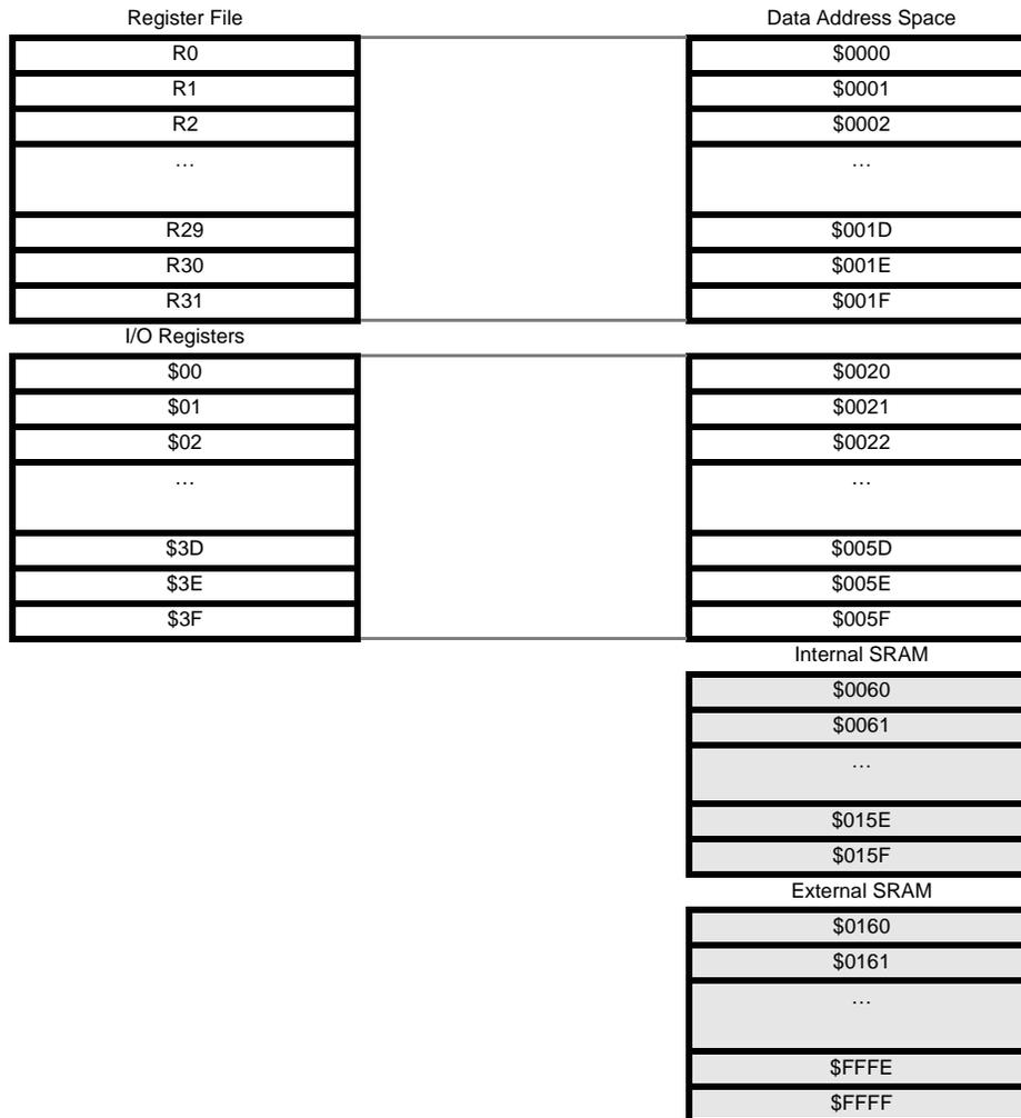
The lower 352 Data Memory locations address the Register file, the I/O Memory and the internal data SRAM. The first 96 locations address the Register File + I/O Memory, and the next 256 locations address the internal data SRAM. An optional external data SRAM can be placed in the same SRAM memory space. This SRAM will occupy
