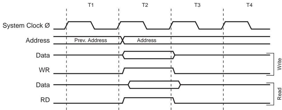
The external data SRAM access is performed in two System Clock cycles as described in Figure 22.
