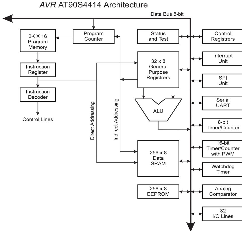
The ALU supports arithmetic and logic functions between registers or between a constant and a register. Single register operations are also executed in the ALU. Figure 4 shows the AT90S4414 AVR Enhanced RISC microcontroller architecture.
