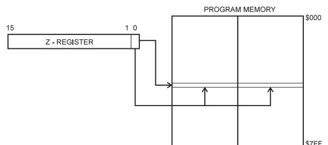
Constant byte address is specified by the Z-register contents. The 15 MSBs select word address (0 - 2K) and LSB, select low byte if cleared (LSB = 0) or high byte if set (LSB = 1).
