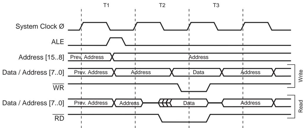
The external data SRAM memory access cycle with the Wait State bit enabled (Wait State active) is shown in Figure 24.
