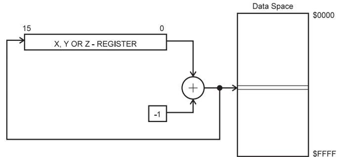
The X, Y or the Z-register is decremented before the operation. Operand address is the decremented contents of the X, Y or the Z-register.
