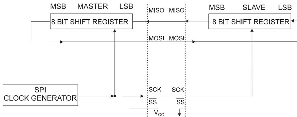
The system is single buffered in the transmit direction and double buffered in the receive direction. This means that characters to be transmitted cannot be written to the SPI Data Register before the entire shift cycle is completed. When receiving data, however, a received character must be read from the SPI Data Register before the next character has been completely shifted in. Otherwise, the first character is lost.
