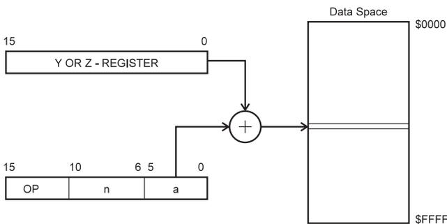
Operand address is the result of the Y or Z-register contents added to the address contained in 6 bits of the instruction word.
