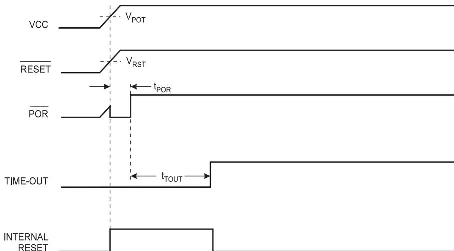
Figure 27. MCU Start-Up,  $\overline{\text{RESET}}$  Tied to  $V_{CC}$ . Slowly Rising  $V_{CC}$
