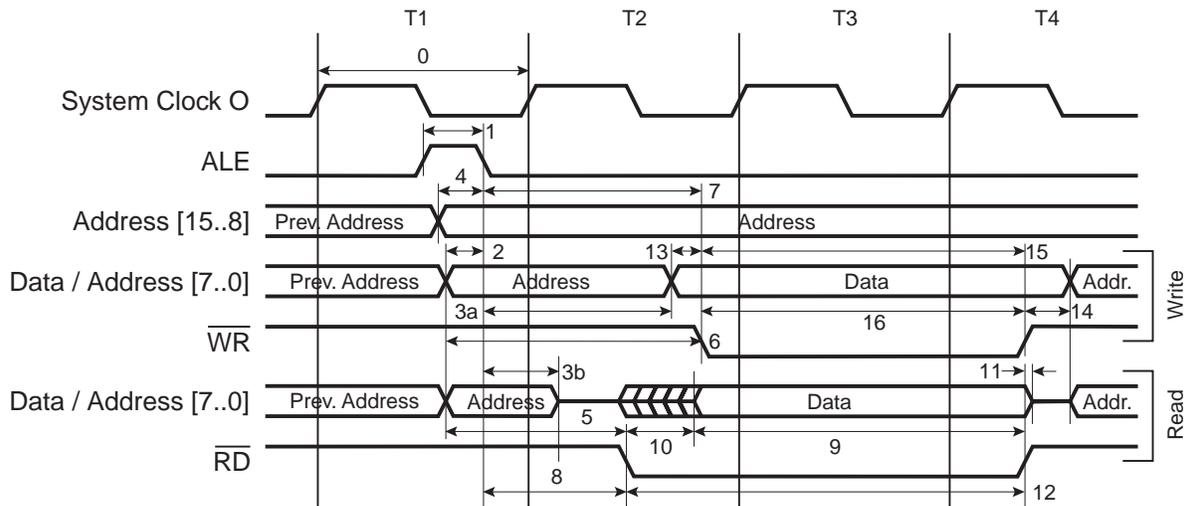
Note: Clock cycle T3 is only present when external SRAM waitstate is enabled
