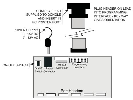
A power supply is required with a standard 2.1mm barrel connector. It can be AC (7 - 12V) or DC (9 - 15V). The connector is inserted into the power connection socket as shown, above.
