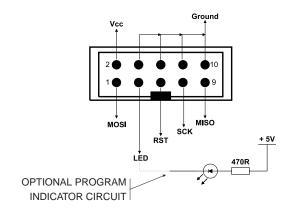
Note: This is a view of the header needed on user circuit, not a face view of ISP lead.
