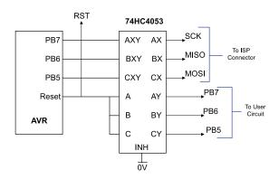
The multiplexer select can be driven from the LED connection on the programming lead as can a low power LED with its cathode connected to the LED connection via a suitable resistor— $1K\Omega$  is fine. If you use this connection then the output will be low 0 during programming and a 1 at all other times. Note that it will float if the programmer is not active, i.e. the software is not running so you may need to use a pull-up resistor.
