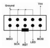
**Note:** This is a face view of the ISP lead. Section 9.2 shows connector on user circuit.
