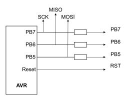
Typical resistor values would be 1K. This circuit is fine if ports PB7, PB6 and PB5 are used as inputs in your circuit. If Outputs are needed, especially higher than a few milliamps, then the multiplexed circuit is preferable.
