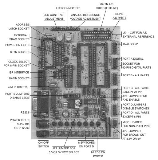
**Note:** There are a number of jumpers on the board which are used to select different operations and voltages. The default jumper settings are for programming operations at 5V. To carry out other operations, some jumpers may have to be removed - refer to the relevant section for details. A full list of the jumpers and links are given in Section 3.1.
