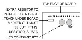
If you use a different LCD driver, it may have a different voltage contrast range. In order to accommodate this, add a resistor to the board, shown above, and cut track on underside of board—marked cut.
