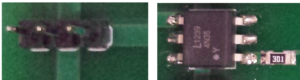
Figure 14: The left image shows the servo pin header used to connect the gimbal servos. The right image shows the optical isolation chip used to electrically isolate the servo control lines from the micro-controller control lines. Each servo output line has one optical isolator and one servo pin header.
