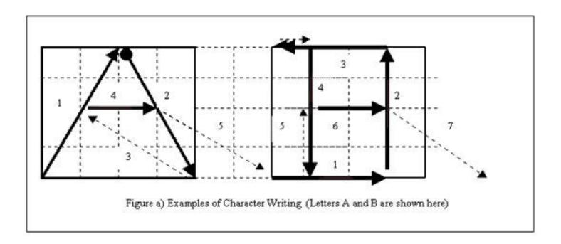
The plotter can also write the 26 English characters in upper case, and the numbers 0-9. Each character/number is break into strokes. The character is put into a 4X4 square, so that the beginning and the end of each stroke is given a coordinate. Here is how we implement the character writing:
