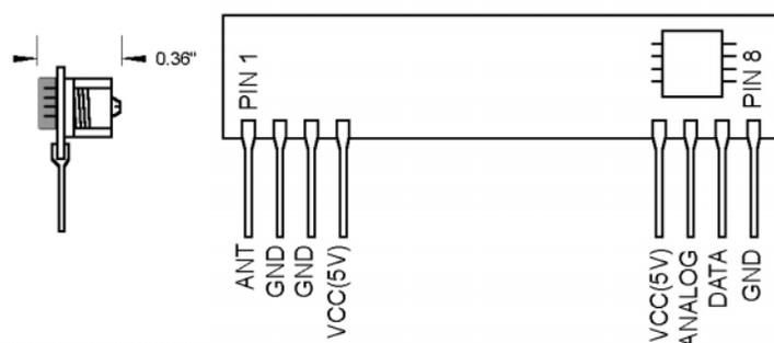
Figure 2. Pin-Out Diagram
