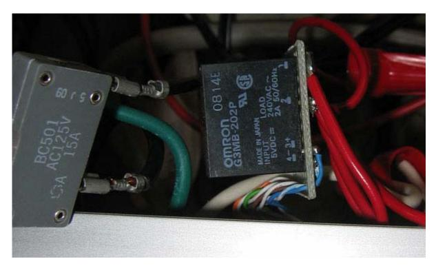
The circuit breaker on the left protected the rest of the world in case something within the box s relays on the right were hooked to the microcontroller with Cat5 twisted pair cable, and to the or gauge stranded wire.
