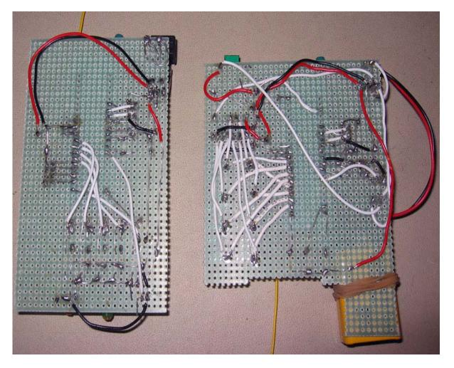
This is the bottom of the two boards. Soldering these two boards was rather tedious and difficu connections are solid and the wires aren't going anywhere. The only real way to neaten it up is printed circuit boards, but that's a little advanced for this early prototyping stage.
