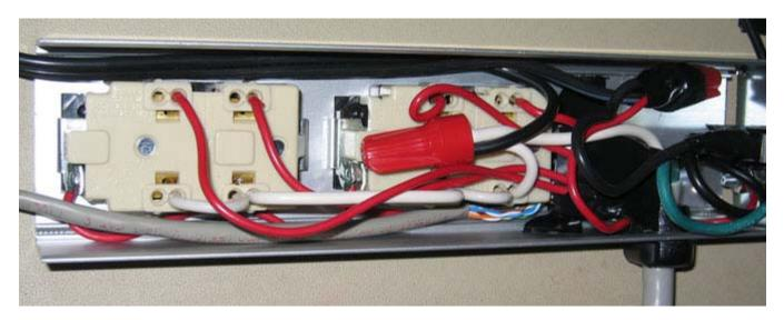
Here's the inside of the strip right before being closed up. There used to be a small switching p jammed in there too, but somehow it blew up. So, instead there's a wire coming out that hooks supply. The relays are covered with electrical tape, right next to the main wire bundle. Interest earth ground wires of the outlets weren't initially hooked to anything, but we fixed that.
