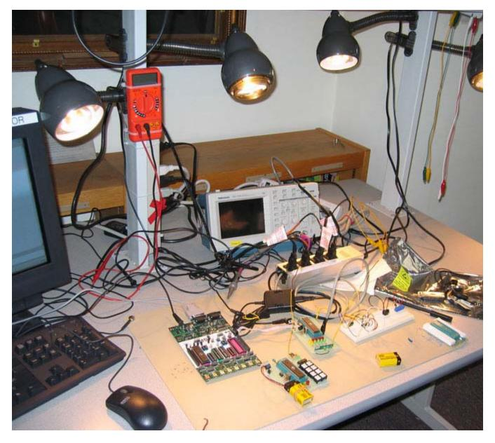
Here's a shot of it all put together. The STK500 is hooked up for programming, and there's a bit to test out some new wacky circuit. We used the 60W lamps in the lab to test the outlets' functi were easy to come by, and made a good display of the project's capabilities.
