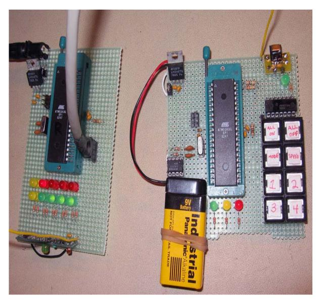
Here are the two circuit boards, transmitter on right and receiver on left. Both used a 17cm piec antenna.
