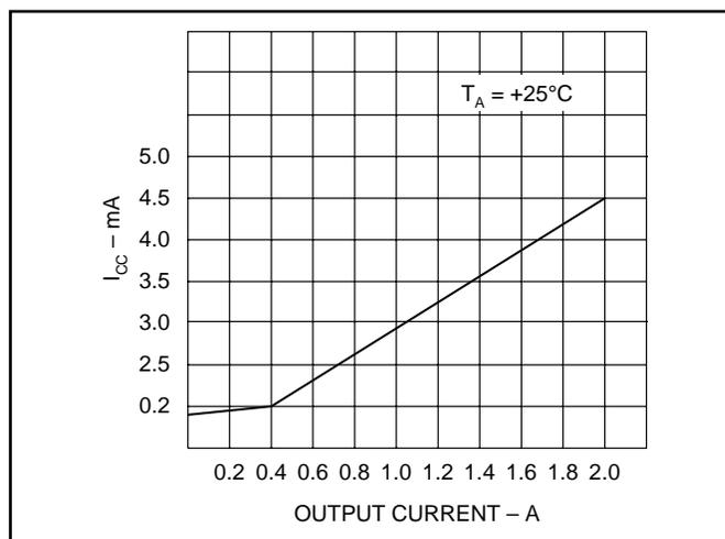
Figure 3. Typical supply current vs. load current.
