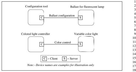
Figure 5.1 Typical Usage of Ballast Configuration and Color Control Clusters
