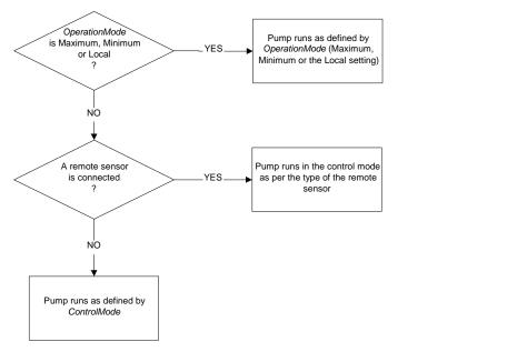
Figure 6.3 Priority Scheme of Pump Operation and Control
