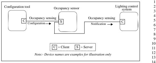
Figure 4.3 Typical Usage of Occupancy Sensing Cluster
