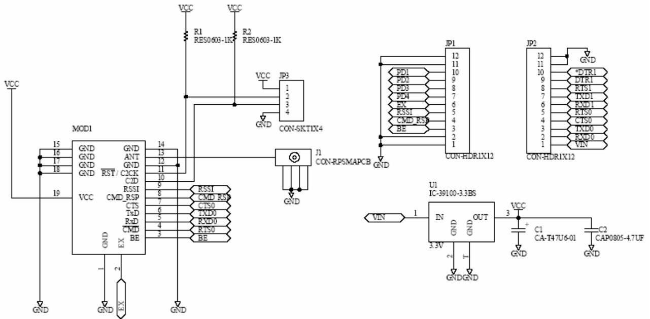
Figure 10: WI.232FHSS-25-FCC-R™ Schematic Diagram
