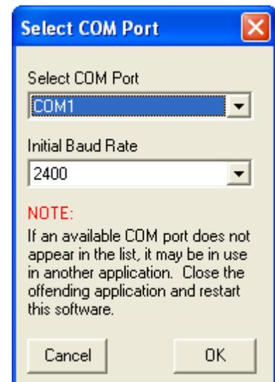
Figure 2: COM Port Setup
