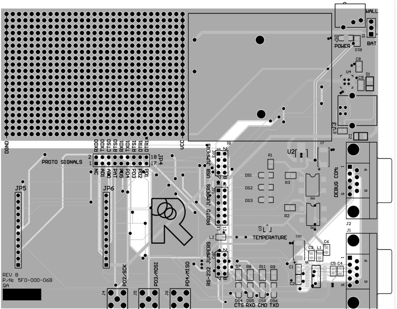
Figure 8: Evaluation Board Layout
