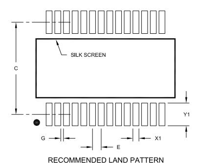
MILLIMETERS Units NOM MAX **Dimension Limits** MIN Contact Pitch 0.65 BSC Ε Contact Pad Spacing С 7.20 Contact Pad Width (X28) X1 0.45 Contact Pad Length (X28) <u>Y1</u> 1.75 Distance Between Pads G 0.20
