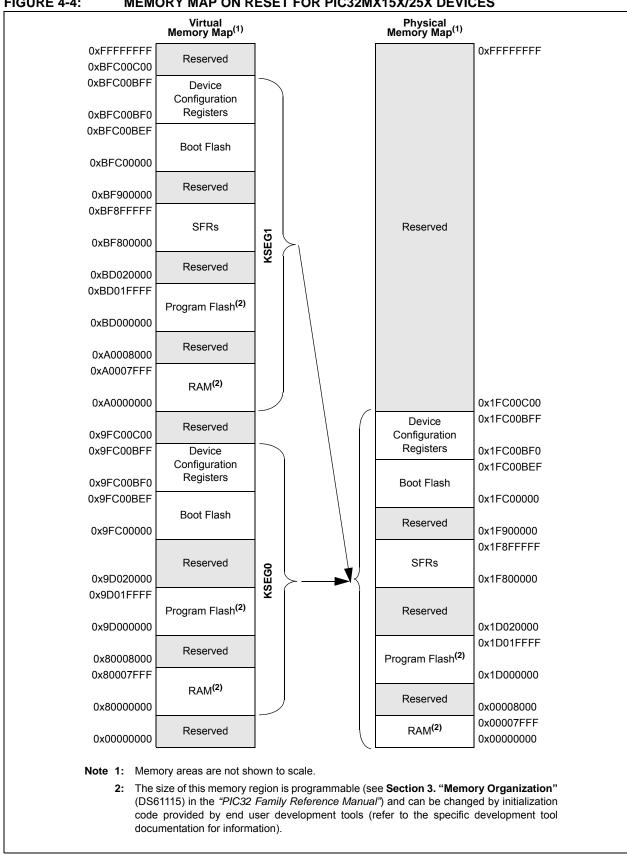
FIGURE 4-4: MEMORY MAP ON RESET FOR PIC32MX15X/25X DEVICES
