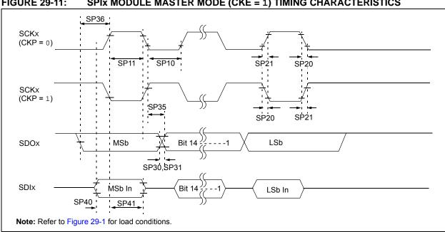
SPIx MODULE MASTER MODE (CKE = 1) TIMING CHARACTERISTICS FIGURE 29-11:
