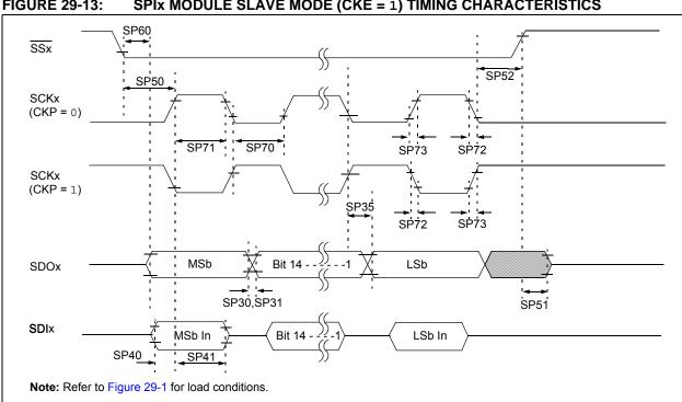
SPIX MODULE SLAVE MODE (CKE = 1) TIMING CHARACTERISTICS FIGURE 29-13:
