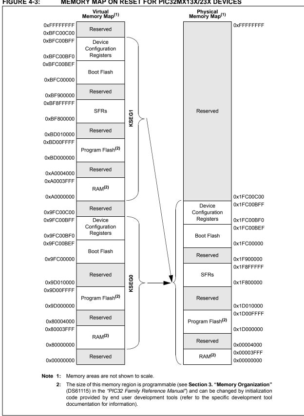
FIGURE 4-3: **MEMORY MAP ON RESET FOR PIC32MX13X/23X DEVICES**
