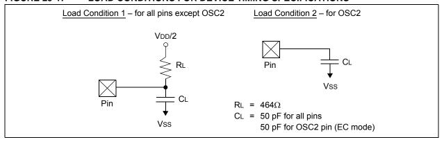
TABLE 29-14: CAPACITIVE LOADING REQUIREMENTS ON OUTPUT PINS
