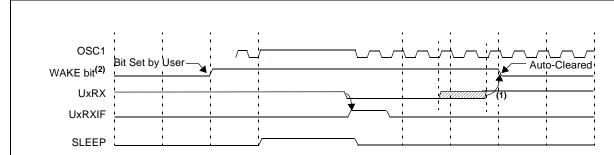
Note 1: If the wake-up event requires long oscillator warm-up time, the auto-clear of the WAKE bit can occur while the system clocks are still active. This sequence should not depend on the presence of Q clocks.
