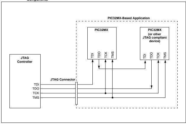
In PIC32MX family devices, the hardware for the JTAG boundary scan is implemented as a peripheral module (i.e., outside of the CPU core) with additional integrated logic in all I/O ports. A logical block diagram of the JTAG module is shown in Figure 33-4. It consists of the following key elements:
