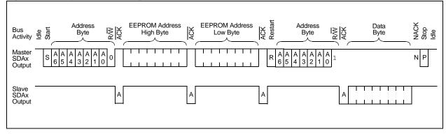
The  $I^2C$  module supports Master mode communication with the inclusion of Start and Stop generators, data byte transmission, data byte reception, an Acknowledge generator and a Baud Rate Generator. Generally, the software will write to a control register to start a particular step, then wait for an interrupt or poll status to wait for completion.
