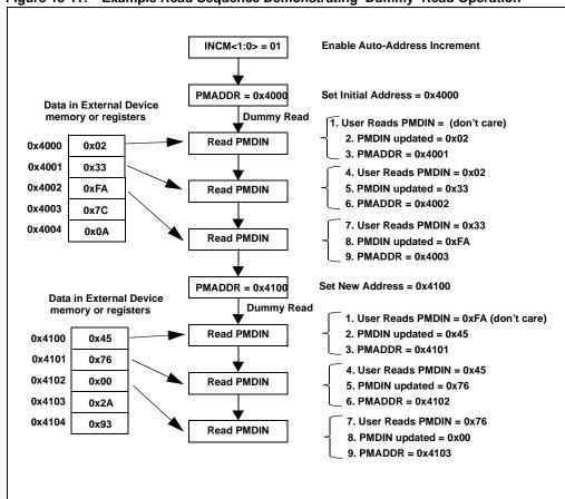
Figure 13-11: Example Read Sequence Demonstrating 'Dummy' Read Operation
