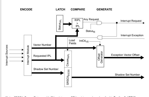
Note: SRSCtl, Cause, Status, and IntCtl registers are CPU registers and are described in Section 2. "CPU".
