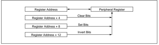
The base register address provides normal Read/Write access, the other three provide special write-only functions.
