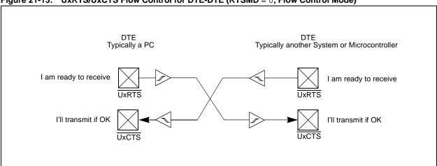
Figure 21-13: UxRTS/UxCTS Flow Control for DTE-DTE (RTSMD = 0, Flow Control Mode)
