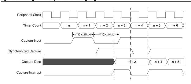
Figure 15-7: Edge Detect Capture Event Timing Diagram
