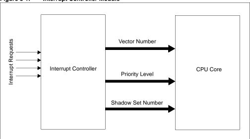
**Note:** Several of the registers cited in this section are not in the interrupt controller module. These registers (and bits) are associated with the CPU. Details about them is available in **Section 2. "MCU".**
