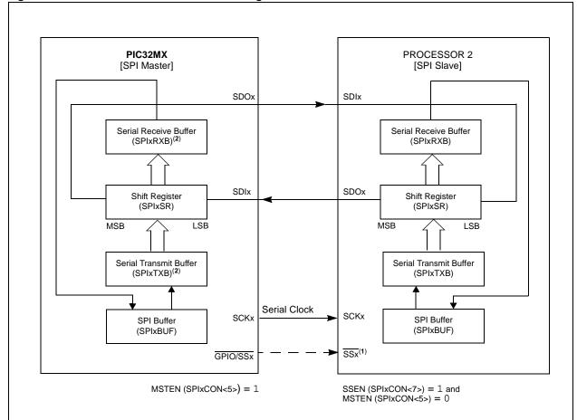
**Note 1:** Using the  $\overline{SSx}$  pin in Slave mode of operation is optional.
