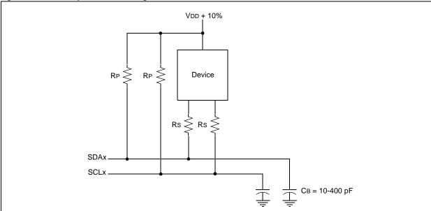
Note: I<sup>2</sup>C<sup>™</sup> devices with input levels related to VDD must have one common supply line to which the pull-up resistor is also connected.
