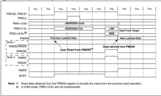
Figure 13-17: 8-Bit, 16-Bit Read Operations, ADRMUX = 01, No Wait States
