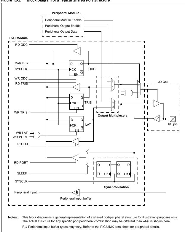
**Block Diagram of a Typical Shared Port Structure**
