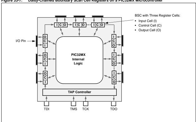
Daisy-Chained Boundary Scan Cell Registers on a PIC32MX Microcontroller Figure 33-7:
