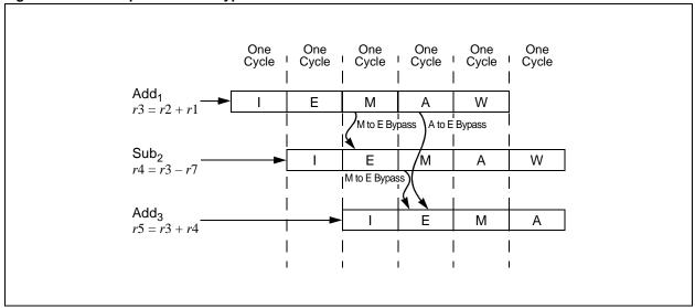
Figure 2-7: IU Pipeline A to E Data Bypass
