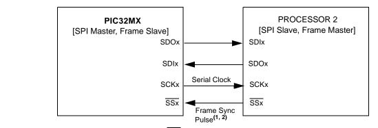
Note 1: In Framed SPI modes, the SSx pin is used to transmit/receive the frame synchronization pulse.
