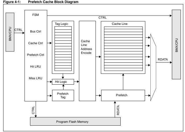
To illustrate the basic operation of the prefetch cache, Figure 4-2 shows an example of the CPU requesting data from physical address 0x1FC01234. The prefetch cache simultaneously compares this address to all of the tags marked "valid". Since the shaded entry below has this address, and is marked as valid, this is a cache hit. The proper data word from the data array is then directed to the CPU in a single clock period.
