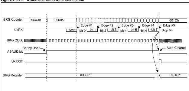
Figure 21-11: Automatic Baud Rate Calculation
