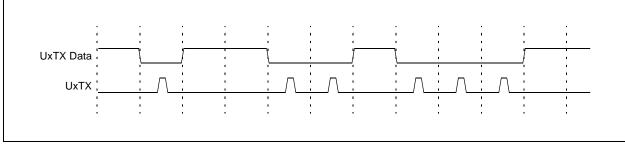
Figure 21-17: IrDA® Encode Scheme for '0' Bit Data
