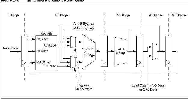
The results of using instruction pipelining in the PIC32MX core is a fast, single-cycle instruction execution environment.
