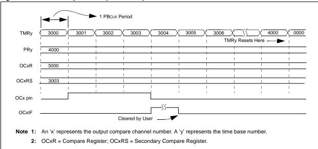
Figure 16-11: Dual Compare Mode (32-Bit Mode)
