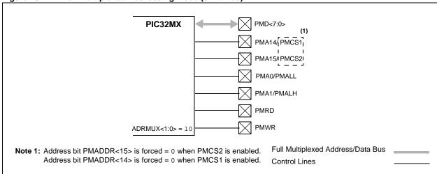
Figure 13-8: Full Multiplexed Address Example (8-Bit Bus)
