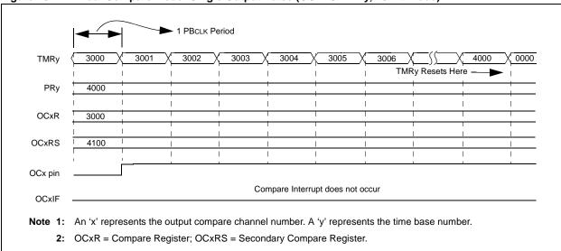
Figure 16-13: Dual Compare Mode: Single Output Pulse (OCxRS > PRy, 32-Bit Mode)
