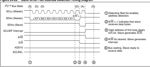
Figure 24-22: Slave Write 7-Bit Address Detection Timing Diagram
