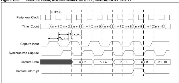
Figure 15-8: Interrupt Event, ICxCON.ICxM<2:0> = 011, ICxCON.ICxI<1:0> = 11
