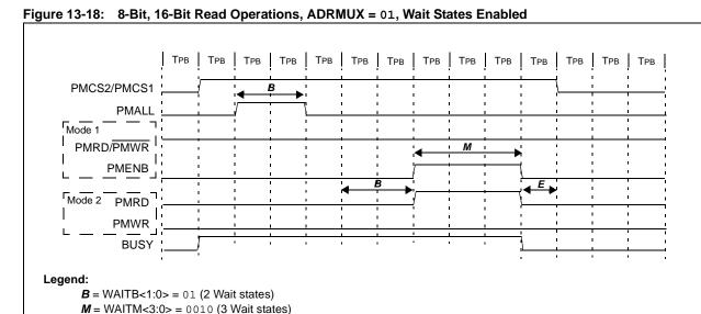
Note: If WAITM<3:0> = 0000, M is forced to 1 T<sub>PBCLK</sub>, WAITB is ignored (B forced to 1 T<sub>PBCLK</sub>) and WAITE is ignored (E forced
