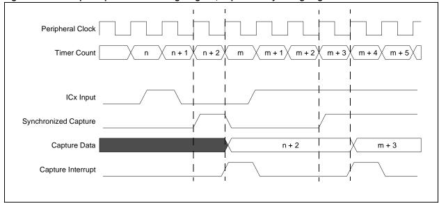
Figure 15-4 depicts a capture event when the Input Capture module is in Simple Capture mode configured to capture every falling edge, ICM = 010 (ICxCON<2:0>), with interrupts generated for every event, ICI = 00 (ICxCON<6:5>). In this example, the timer frequency is slower than the peripheral clock.
