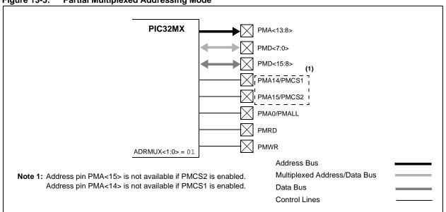
Figure 13-6: Partial Multiplexed Addressing Example
