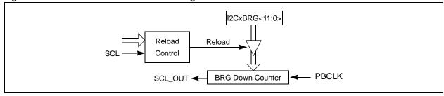
Figure 24-6: Baud Rate Generator Timing With Clock Arbitration
