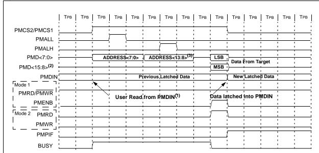
Figure 13-21: 8-Bit, 16-Bit Read Operations, ADRMUX = 10, No Wait States
