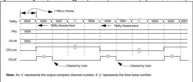
Figure 16-9: Single Compare Mode: Toggle Output on Compare Match Event (PRy = OCxR, 32-Bit Mode)
