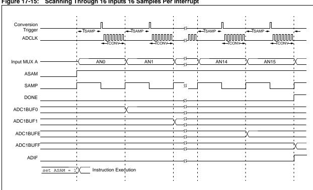
Figure 17-15: Scanning Through 16 Inputs 16 Samples Per Interrupt
