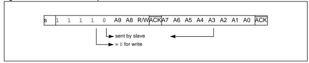
Figure 24-25: 10-Bit Address Detection Timing Diagram
