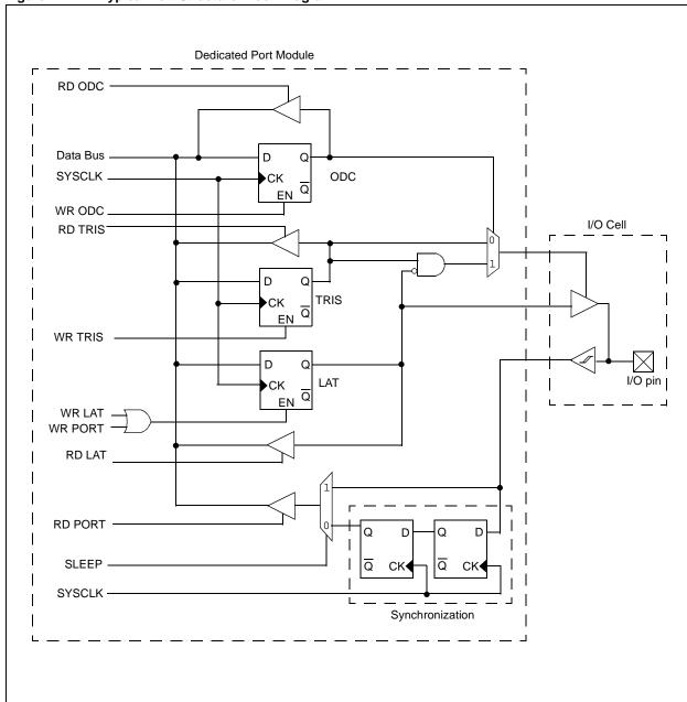
Figure 12-1: Typical Port Structure Block Diagram
