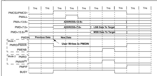
**Note 1:** During a write operation, there is one TPBCLK hold cycle following the PMWR signal.
