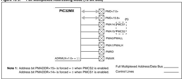
Figure 13-10: Full Multiplexed Addressing Example (16-Bit Bus)
