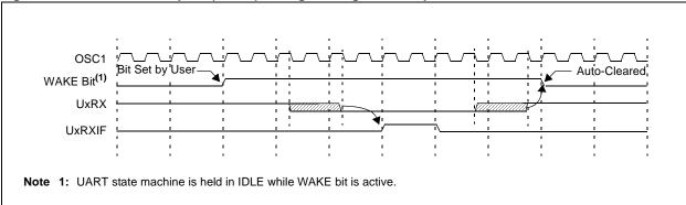
Figure 21-23: Auto-Wake-up Bit (WAKE) Timings During SLEEP
