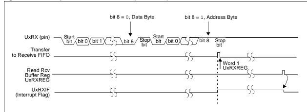
Note: This timing diagram shows a data byte followed by an address byte. The data byte is not read into the UxRXREG (receive buffer) because ADDEN = 1 and bit 8 = 0.
