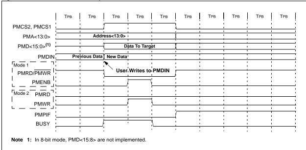
In this timing diagram with Wait states, the write operation requires 7  $T_{PBCLK}$ , peripheral-bus-clock cycles.
