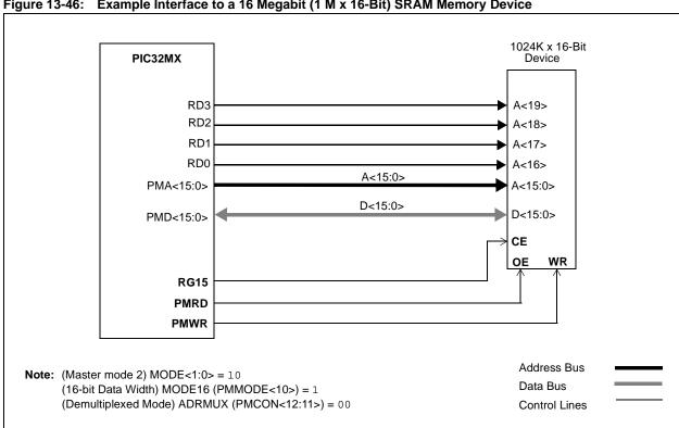
Example Interface to a 16 Megabit (1 M x 16-Bit) SRAM Memory Device
