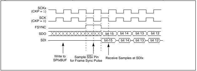
Figure 23-13: SPI Master, Frame Slave Connection Diagram
