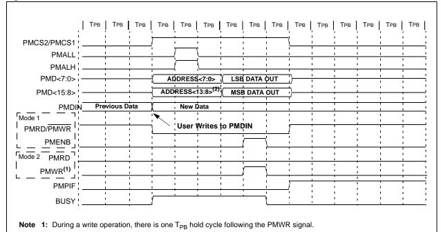
2: PMADDR Address bit A15 and A14 are forced to '0' if PMCS2 and/or PMCS1 are enabled as Chip Selects.
