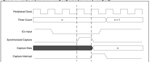
Figure 15-5 depicts a capture event when the Input Capture module is in Simple Capture mode configured to capture every edge, ICM = 011 (ICxCON<2:0>); starting with a falling edge, ICFEDGE = 0 (ICxCON<9>), with interrupts generated for every second event, ICI = 01 (ICxCON<6:5>).
