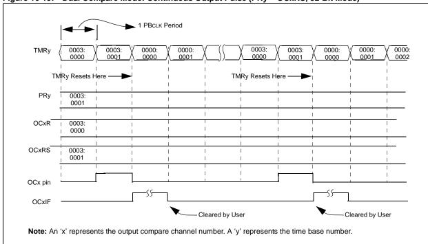
Figure 16-16: Dual Compare Mode: Continuous Output Pulse (PRy = OCxRS, 16-Bit Mode)
