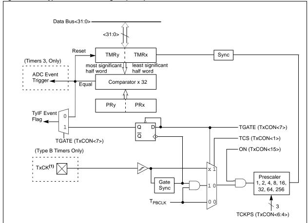
Note 1: In certain variants of the PIC32MX family, the TxCK pin may not be available. Refer to the device data sheet for the I/O pin details. In such cases, the timer must use the peripheral clock as its input clock.
