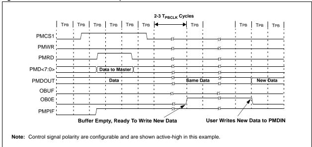
Figure 13-35: Parallel Slave Port Read Operation – Buffer Empty, Underflow Condition
