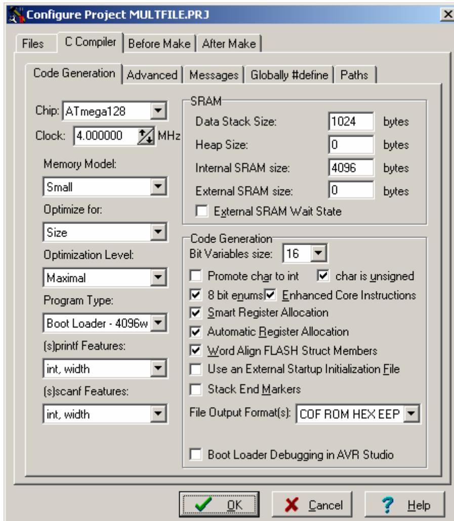
If this option is enabled, the compiler will generate supplementary code that allows the Boot Loader to be source level debugged in the AVR Studio simulator/emulator.
