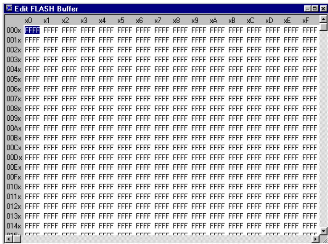
The buffer's contents, at the highlighted address, can be edited by pressing the **F2** key and typing in the new value. The edited value is saved by pressing the **Tab** or **arrow** keys.
