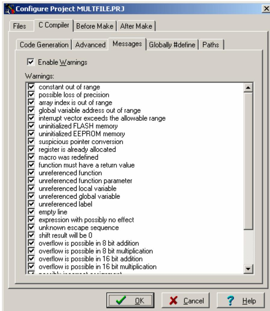
The generation of warning messages during compilation can be globally enabled or disabled by using the **Enable Warnings** check box.
