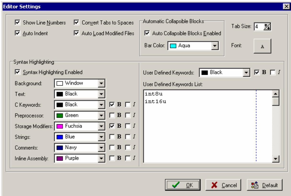
The **Show Line Numbers** check box, allows enabling or disabling the displaying of line numbers in the Editor windows.
