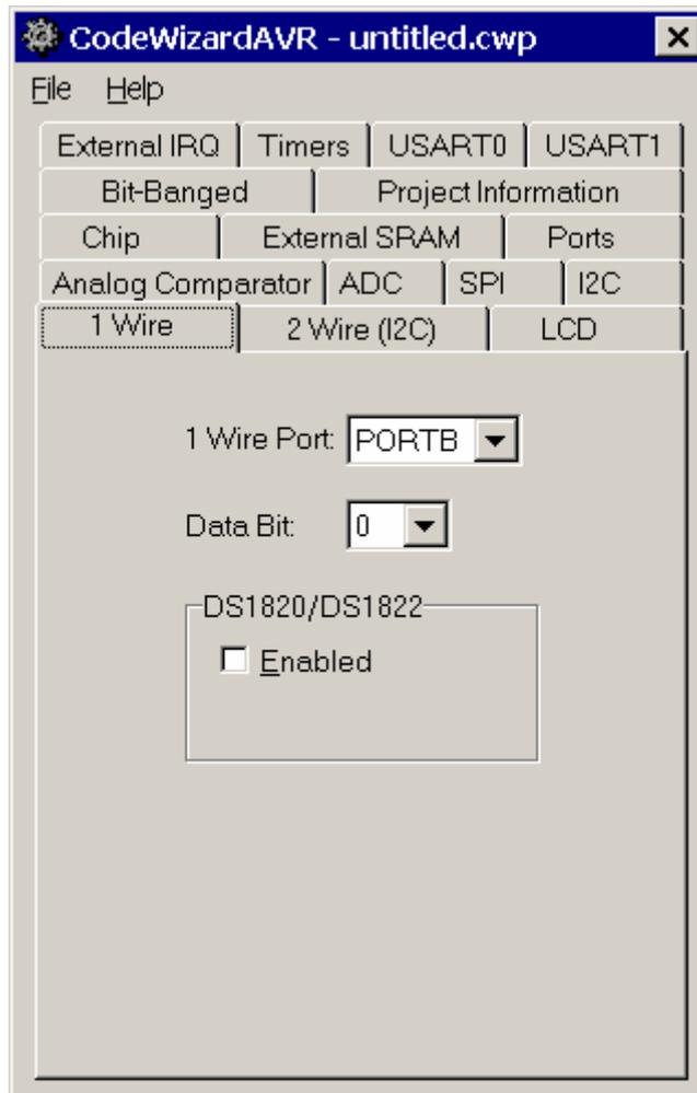
Using the **1 Wire Port** list box you can specify which port is used for the implementation of the 1 Wire bus.
