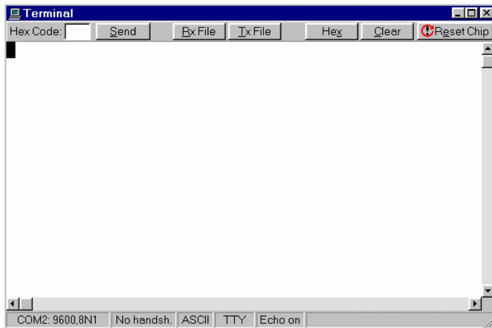
The characters can be displayed in ASCII or hexadecimal format. The display mode can be toggled using the **Hex/ASCII** button.
