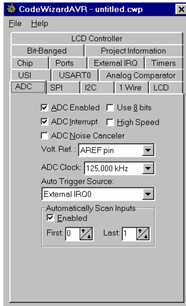
Checking the **ADC Enabled** check box enables the on-chip ADC.
