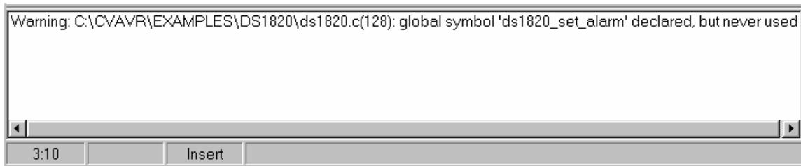
By double clicking on the error or warning message, the line with the problem will be highlighted. The size of the **Message** window can be modified using the horizontal slider bar placed between it and the **Editor** window.
