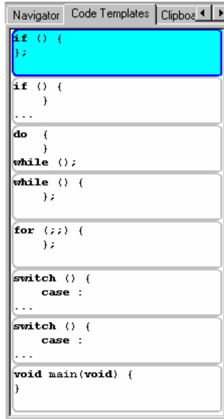
This is achieved by clicking on the desired code sequence in the Code Templates window and then dragging and dropping it to the appropriate position in the Editor window.
