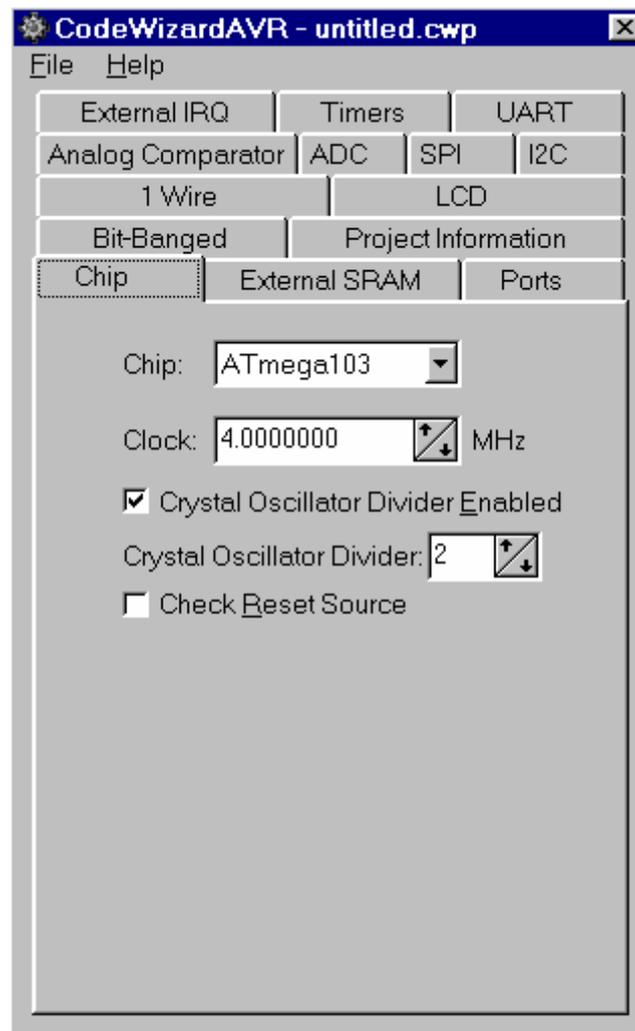
The chip type can be specified using the **Chip** list box.
