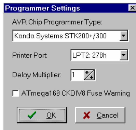
The **Delay Multiplier** value can be increased in case of programming problems on very fast machines. Of course this will increase overall programming time.
