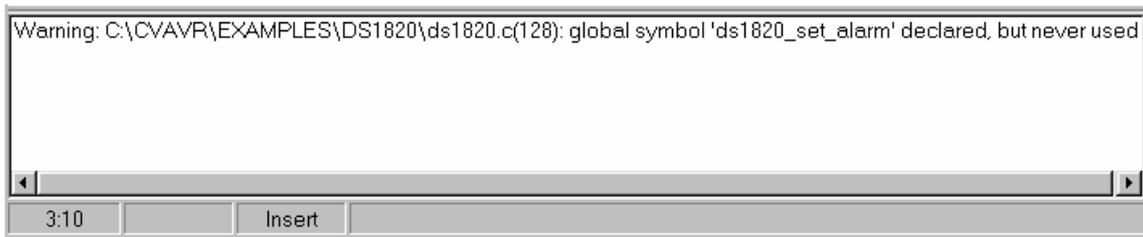
By double clicking on the error or warning message, the line with the problem will be highlighted. If no errors were encountered, then the Atmel AVR assembler AVRASM32 will be executed, obtaining the output file type specified in **Project|Configure|C Compiler|Code Generation**.
