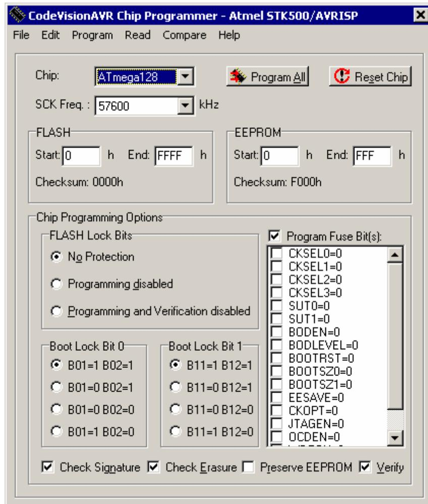
You can select the type of the chip you wish to program using the **Chip** combo box.
