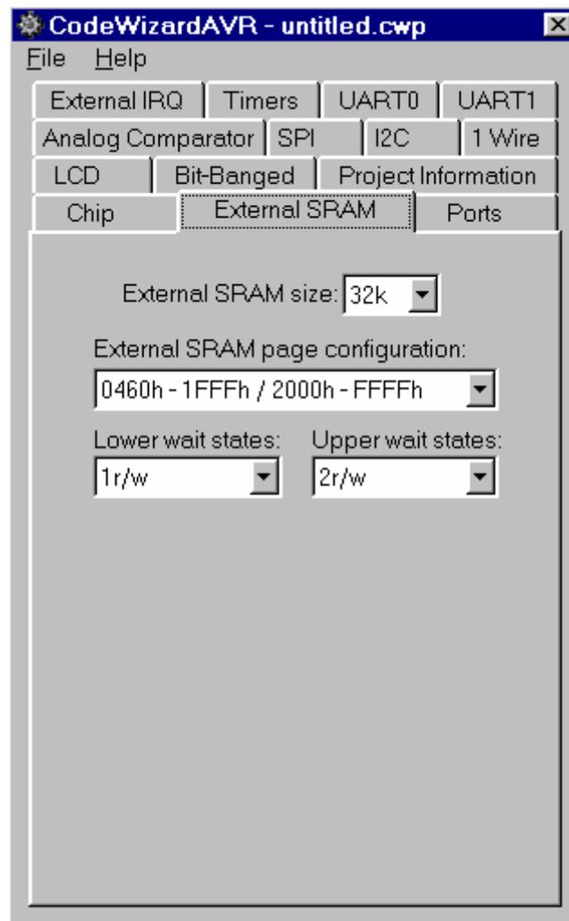
The **External SRAM page configuration** list box allows selection of the splitting address for the two external SRAM pages .
