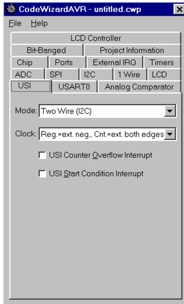
The **Shift Reg. Clock** list box sets the clock source for the USI Shift Register and Counter.
