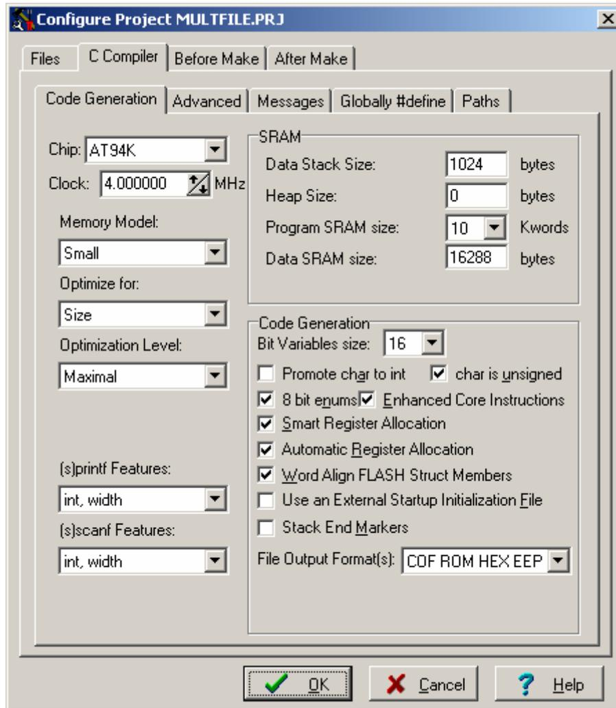
The maximum size of the global bit variables, which are placed in the GPIOR (if present) and registers R2 to R14, can be specified using the **Bit Variables size** list box.
