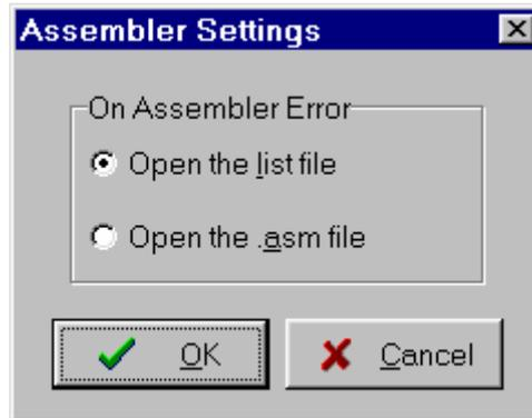
The **On Assembler Error** options allow to select which file will be automatically opened by the **Editor** in the case of an assembly error.
