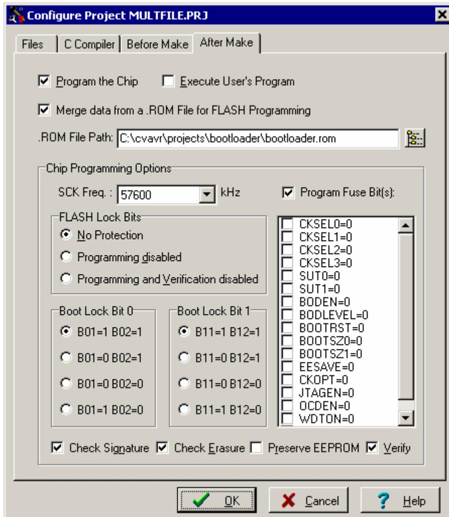
If you check the **Program the Chip** option, then after successful compilation/assembly your program will be automatically transferred to the AVR chip using the built-in Programmer software.
