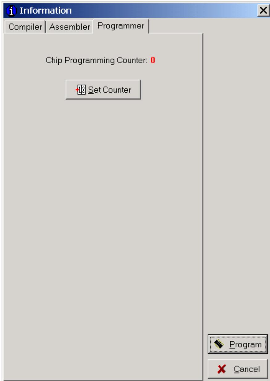
Pressing the **Set Counter** button will open the **Set Programming Counter** window:
