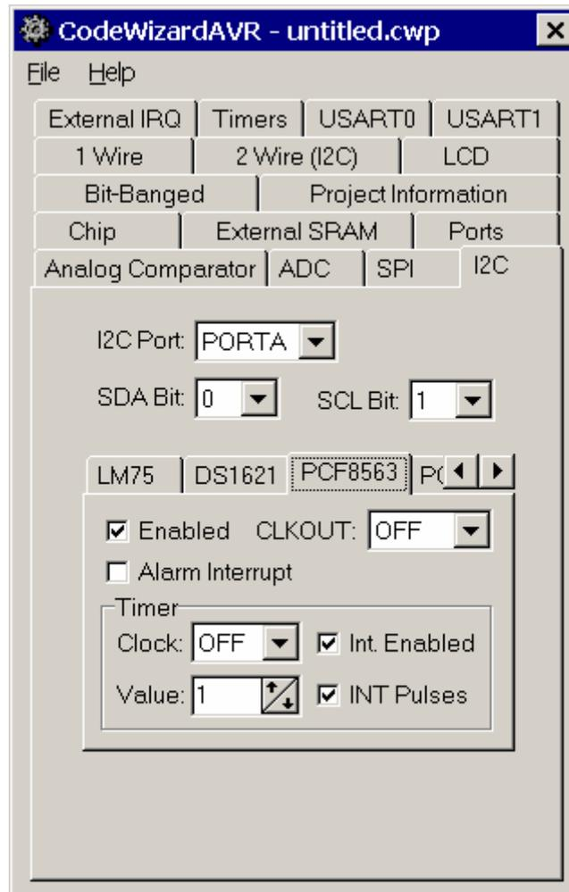
The **CLKOUT** list box specifies the frequency of the pulses on the CLKOUT output.
