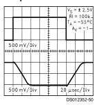
Inverting Large Signal Pulse Response at 5V
