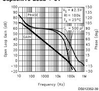
Gain and Phase vs Capacitive Load @ 5V
