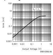
Sourcing Output vs Output Voltage
