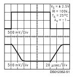
Inverting Large Signal Pulse Response at 5V
