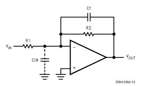
FIGURE 3. Cancelling the Effect of Input Capacitance
