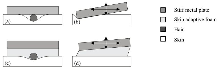
**Figure 2.** Advantages of foam electrodes in comparison to stiff dry electrodes. (a) Loss of contact area and increase of contact impedance due to hairs. (b) Loss of contact and increase of artifacts due to charging effects caused by motion of electrode relative to skin. (c) Increased contact area. (d) Contact maintained during movements.
