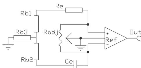
**Figure 5.** Input circuit of the operational amplifier used in the filter electrode setup using only two electrodes. The adjustable resistor  $R_{adj}$  balances the potential instead of using a third electrode as a reference.
