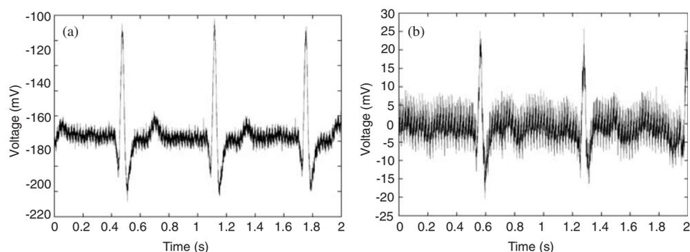
**Figure 17.** (a) Gel electrodes and (b) Ag-SiO<sub>2</sub> electrodes placed next to each other at a selected position. Positioning the electrodes as close as 1 cm from each other still produces a usable signal.
