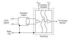
Figure 8. LOC110 Isolated Amplifier in ECG Application
