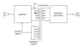
Figure 7A. DC-to-DC Converter with Feedback Winding
