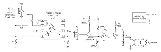
Figure 9B. 0-10V to 4-20mA Converted
