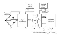
Figure 9. Isolated Pressure Transmitter
