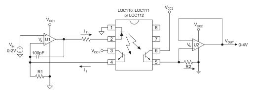
Figure 1. Isolation Amplifier (Photoconductive Operation)
