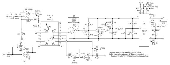
Figure 6. Typical Modem DAA using the LOC210P
