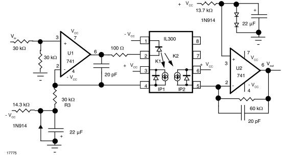
Fig. 24 - Bipolar Photoconductive Isolation Amplifier
