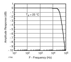
Fig. 12 - Photovoltaic Amplifier Frequency Response
