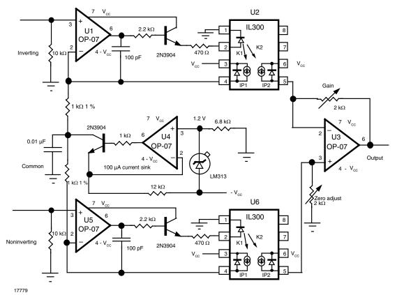
Fig. 28 - Differential Photoconductive Isolation Amplifier
