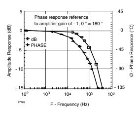
Fig. 31 - Transistor Unipolar Photoconductive Isolation Amplifier Frequency and Phase Response
