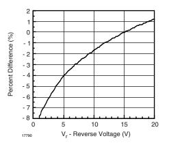
Fig. 40 - Photoconductive Responsivity vs. Bias Voltage The photodiode operated in the photoconductive mode is easily connected to an operational amplifier. Figure 41 shows the diode connected to a trans resistance amplifier. The transfer function of this circuit is given in equation 5a.
