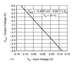
Fig. 29 - Differential Photoconductive Isolation Amplifier Transfer Characteristics
