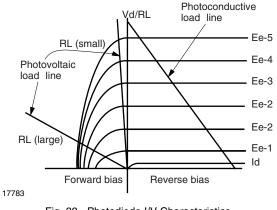
Fig. 33 - Photodiode I/V Characteristics
