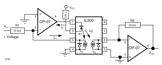
Fig. 10 - Positive Unipolar Photovoltaic Aamplifier
