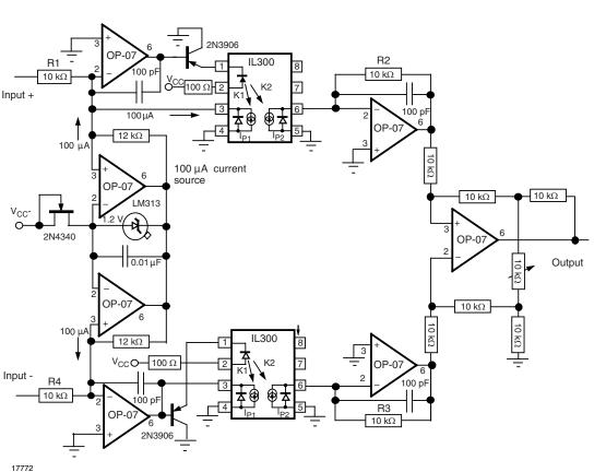
Fig. 21 - Differential Pre Biased Photovoltaic Isolation Amplifier
