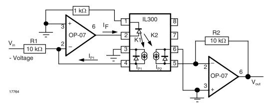
Fig. 13 - Negative Unipolar Photovoltaic Isolation Amplifier
