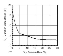
Fig. 42 - Photodiode Junction Capacitance vs. Reverse Voltage
