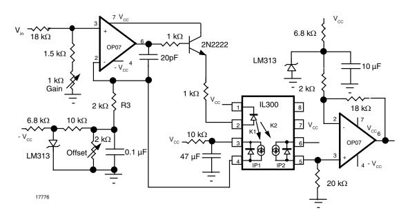
Fig. 25 - High Stability Bipolar Photoconductive Isolation Amplifier
