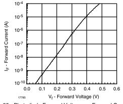
Fig. 35 - Photodiode Forward Voltage vs. Forward Current Inserting the diode equation 2a into the two nodal equations gives the following DC solution for the photovoltaic operation (equation 3a):
