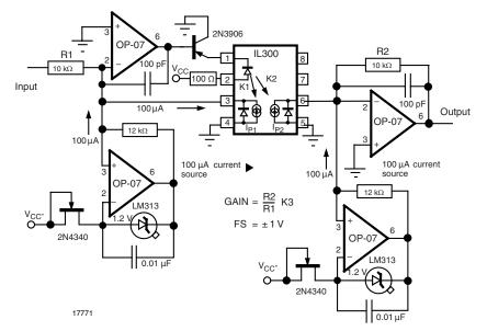
Fig. 20 - Pre Biased Photovoltaic Isolation Amplifier
