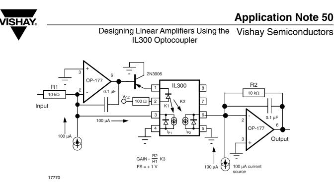
Fig. 18 - Pre Biased Photovoltaic Isolation Amplifier
