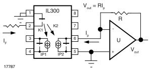
Fig. 37 - Photovoltaic Amplifier Configuration
