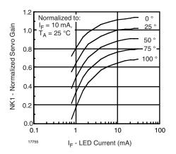
Fig. 4 - Normalized Servo Gain vs. LED Current
