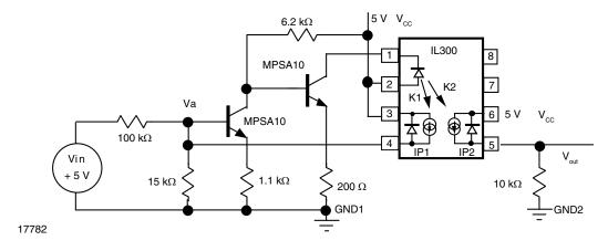
Fig. 32 - Unipolar Photoconductive Isolation Amplifier with Discrete Transistors
