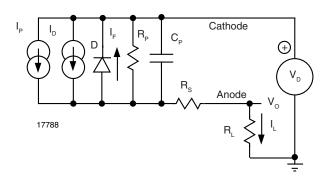
Fig. 38 - Photoconductive Photodiode Model
