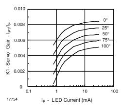
Fig. 3 - Servo Gain vs. LED Current
