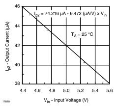
Fig. 30 - Transistor Unipolar Photoconductive Isolation Amplifier Transfer Characteristics
