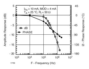
Fig. 43 - Phase and Frequency Response
