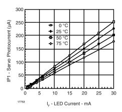
Fig. 2 - Servo Photocurrent vs. LED Current
