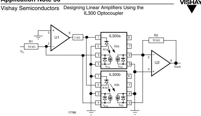
Fig. 15 - Bipolar Input Photovoltaic Isolation Amplifier
