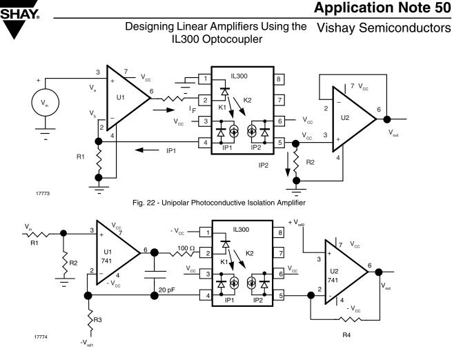
Fig. 23 - Bipolar Photoconductive Isolation Amplifier
