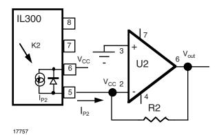
Fig. 6 - Optical Servo Amplifier
