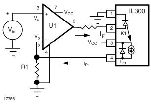
Fig. 5 - Optical Servo Amplifier
