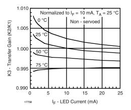
Fig. 7 - Normalized Servo Transfer Gain
