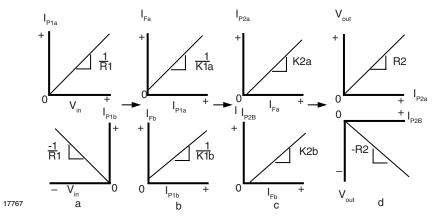
Fig. 16 - Bipolar Input Photovoltaic Isolation Amplifier Transfer Characteristics
