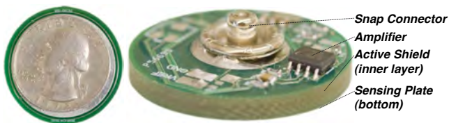
Figure 2: Picture of the non-contact, capacitive electrode. The sensor is manufactured on a standard PCB, which contains the amplifier circuits on the top and the sensing plate on the bottom.
