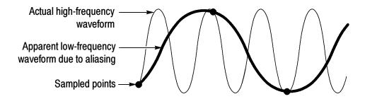
The oscilloscope accurately represents signals, but is limited by the probe bandwidth, the oscilloscope bandwidth, and the sample rate. To avoid aliasing, the oscilloscope must sample the signal more than twice as fast as the highest frequency component of the signal.
