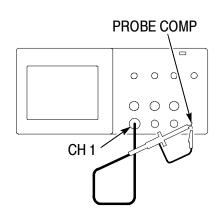
2. Set the switch to 10X on the P2200 probe and connect the probe to channel 1 on the oscilloscope. To do this, align the slot in the probe connector with the key on the CH 1 BNC, push to connect, and twist to the right to lock the probe in place.
