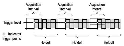
Triggers are not recognized during holdoff time.
