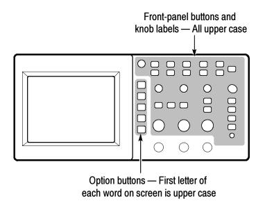
**NOTE**. Option buttons can also be called screen buttons, side-menu buttons, bezel buttons, or soft keys.
