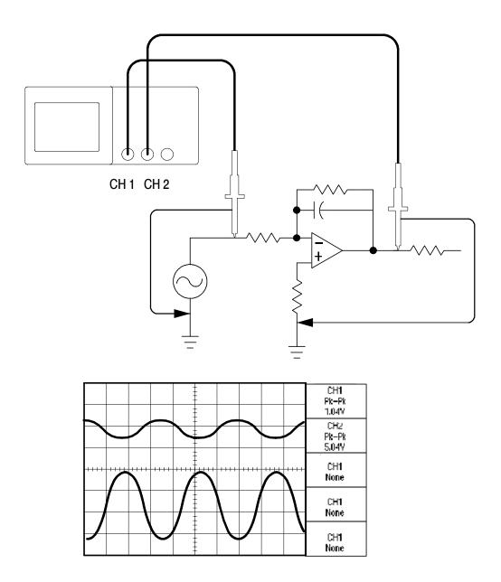
To activate and display the signals connected to channel 1 and to channel 2, follow these steps:
