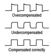
**3.** Check the shape of the displayed waveform.
