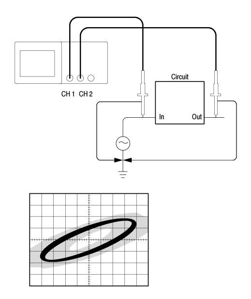
To view the input and output of the circuit in an XY display, follow these steps:
