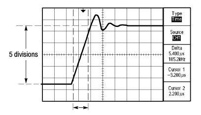
**NOTE**. The Rise Time measurement is available as an automatic measurement in the Measure Menu, described on page 94.
