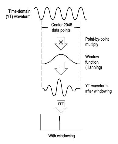
The Math FFT function includes three FFT Window options. There is a trade-off between frequency resolution and amplitude accuracy with each type of window. What you want to measure and your source signal characteristics help you to determine which window to use.
