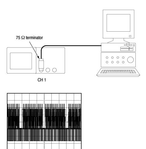
**NOTE**. Most video systems use 75 ohm cabling. The oscilloscope inputs do not properly terminate low impedance cabling. To avoid amplitude inaccuracy from improper loading and reflections, place a 75 ohm feedthrough terminator (Tektronix part number 011-0055-02 or equivalent) between the 75 ohm coaxial cable from the signal source and the oscilloscope BNC input.
