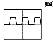
**3.** Push the AUTOSET button. Within a few seconds, you should see a square wave in the display of about 5 V peak-to-peak at 1 kHz.
