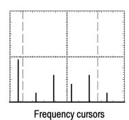
You can also take a frequency measurement. To do so, turn the Horizontal Position knob to position a frequency component on the center graticule line and read the frequency at the top right of the display.
