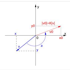
The rotation is a similarity rotation because the magnitude of the produced vector v0 is scaled up by the CORDIC specific constant K( $^{1.646760258121}$ ). The equations of the coordinates for vector v0 are:
