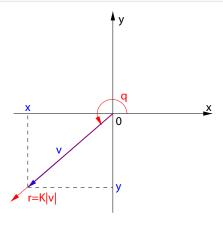
The function takes inputs x and y and outputs a=atan2(y, x) and  $M = K(x^2 + y^2)^{0.5}$ . M is the magnitude of the input vector v=(x,y) $^T$ , scaled by a CORDIC specific constant that converges to 1.646760258121, which
