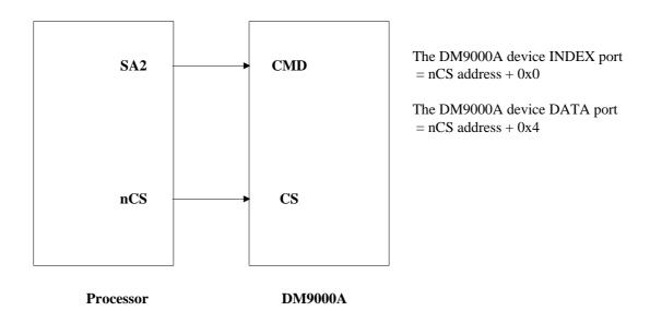
Figure 2.2 CMD Pin and Processor Interface.
