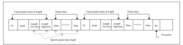
Figure 5.2 Block Diagram of the Received Packets.
