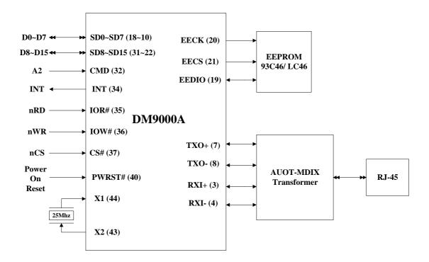
Figure 2.1 Signal Connection with a Processor Interfacing.
