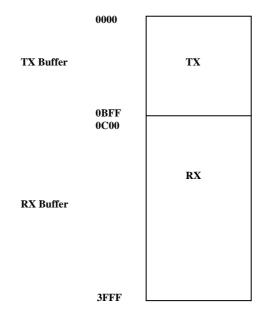
Figure 5.1 Packet Transmitting Buffer.
