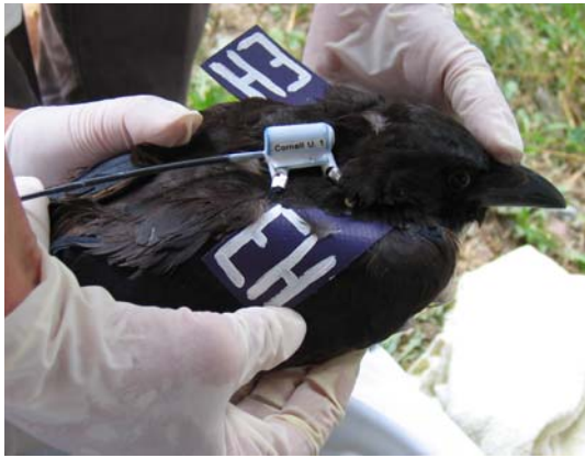
Fig. 4 American Crow with prototype DSSS transmitter
