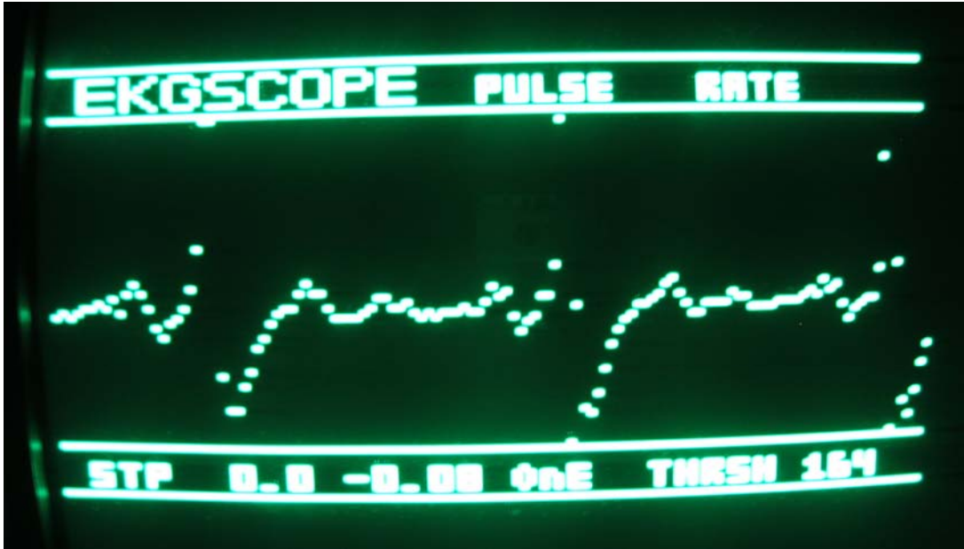
Figure 25: EKG Waveform from receiver shown on our scrolling display
