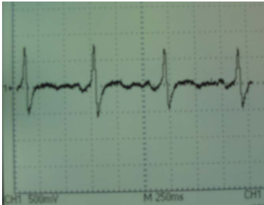
Figure 24: EKG Waveform from receiver shown on a standard oscilloscope
