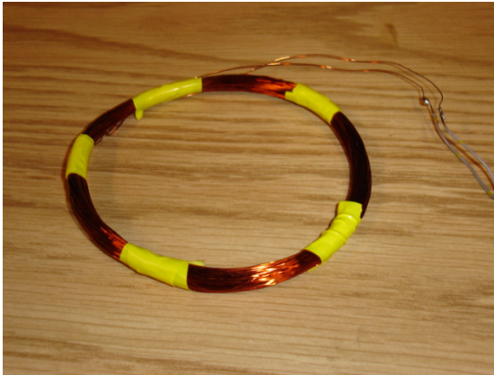
Figure14. Initial Base Station Coil Resonates at ~125 kHz with a 1.1 nF capacitor Diameter: 10cm or 3.9 inches Wire Size: 0.333mm or 0.39 inches No of Turns: 125 Estimated Inductance: 1.625 mH
