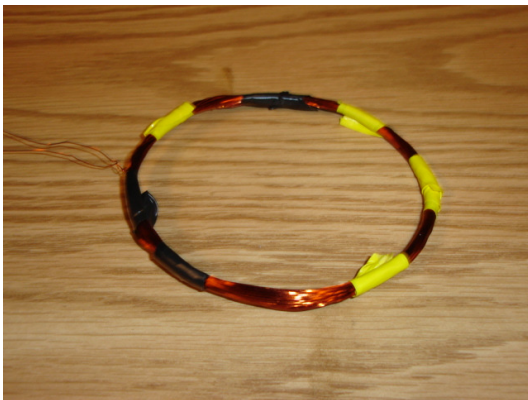
Figure15. Initial Transponder Coil and Final Base Station Coil Resonates at ~125 kHz with a 2.35 nF capacitor Diameter: 10cm or 2.3 inches Wire Size: 0.333mm or 0.39 inches No of Turns: 67 Estimated Inductance: 689 uH
