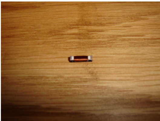
Figure17. Final Ferrite Cored Coil for the Transponder from Coilcraft [10] Resonates at \sim 125 kHz with a 294 nF capacitor
