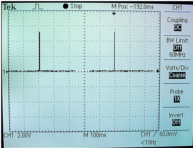
Fig 3: Pulse Frequency when the heart rate is set to 120bpm
