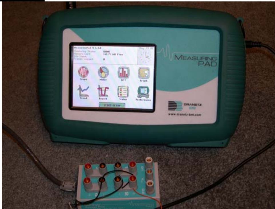
Figure 7 Measuring Pad used for Electrical Characterization
