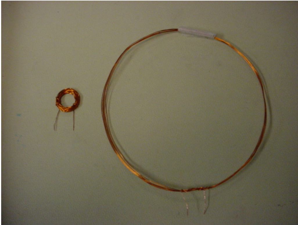
Figure 12: Final Air Core Antennas
