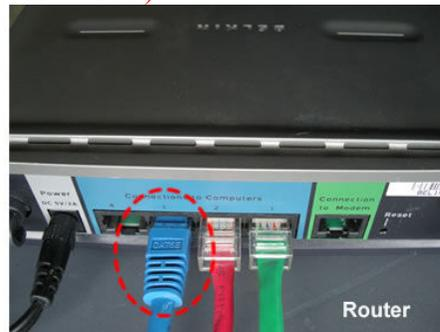
9. Connect a CAT5 RJ45 cable from the “Port A” Port on the Insteon ISY-99i/IR Pro to the Insteon Powerline Modem. ([Universal Devices Tech Support, 818-631-0333](#))
