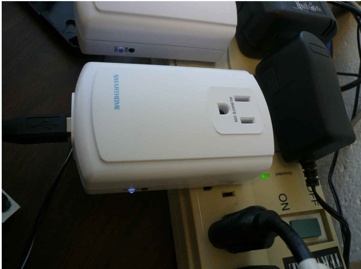
Figure 10: The PowerLinc modem with the LED's on the side that are used for linking purposes
