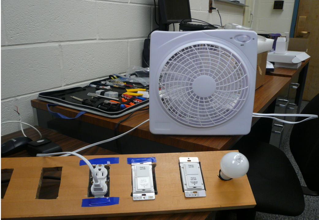
Figure 12: Temporary bench to test SwitchLine Relays connected to a fan via an electrical outlet
