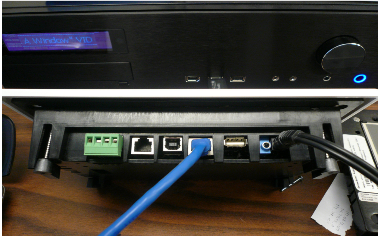
Figure 4: The bottom of the mPanel where the Ethernet cable is to be connected
