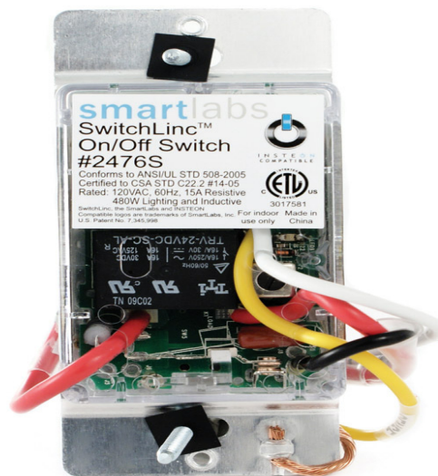
Figure 9: The backside of the SwitchLinc Relay
