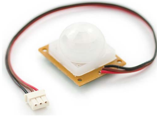
Figure 8-1 Photo of the SE-10 PIR motion sensor
