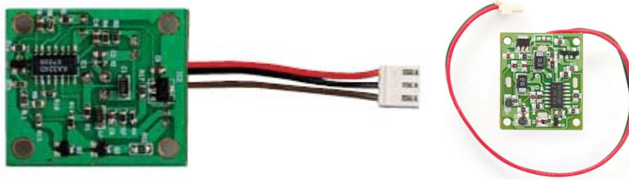
Figure 8-2 Photos of the bottom side of the SE-10 PIR motion sensor
