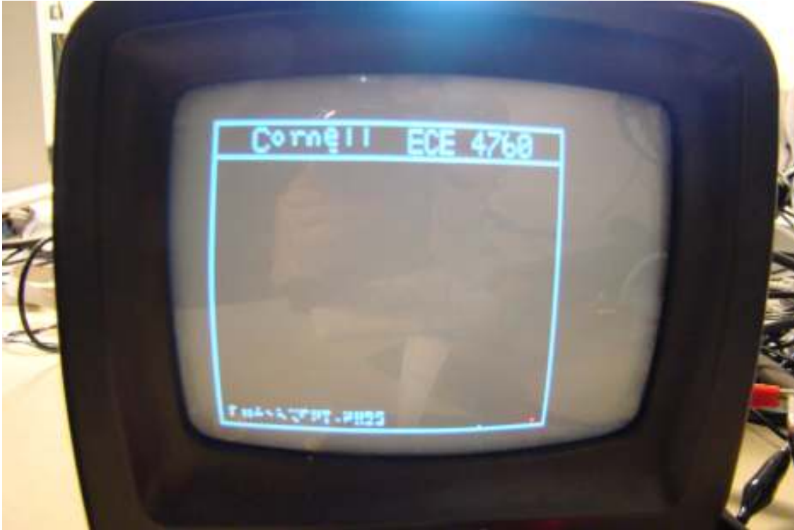
Figure 4: Close-up of screen with ATmega32 code running.
