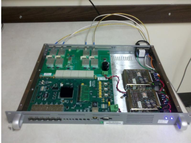
Figure 1. Brookhaven National Laboratory's realized RF Beam Position Monitor, chassis cover removed.
