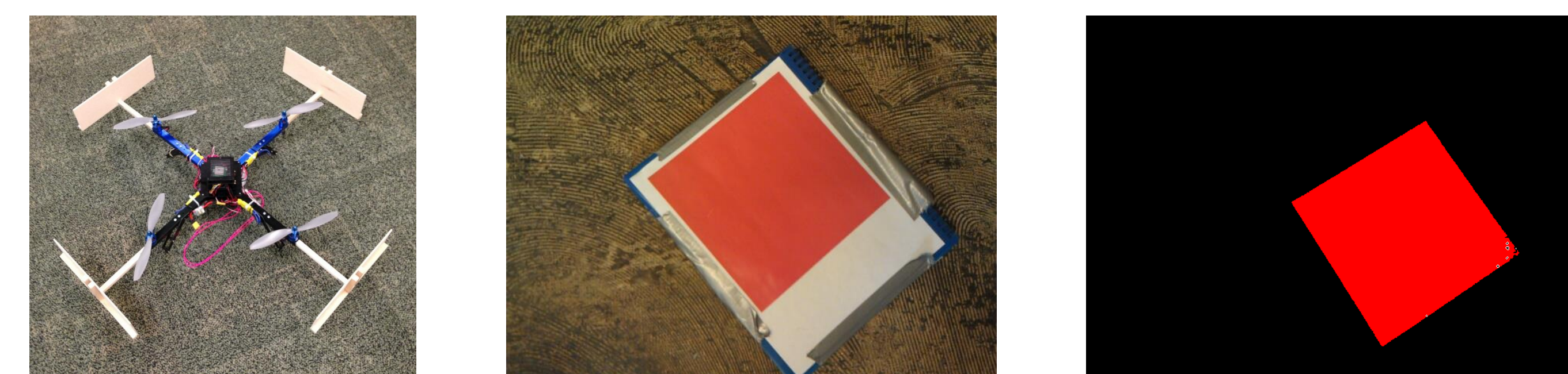
Left: Assembled Quadcopter with propeller protectors. Center: the target. Right: A thresholded image detecting the largest red object.
