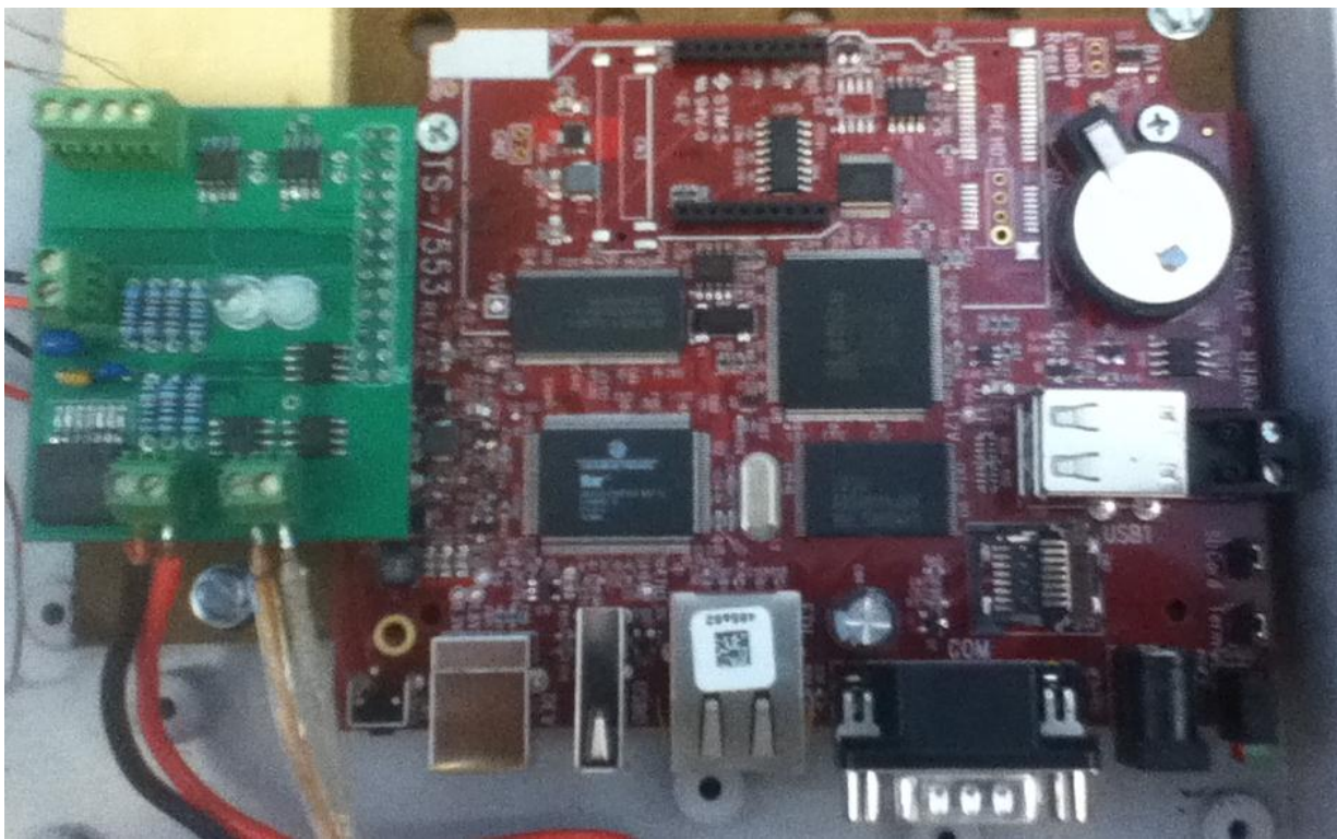
Figure 4: The new webplug. The TS-7553 is on the right (red board), the PCB attachment is mounted onto the TS-7553 (green board).
