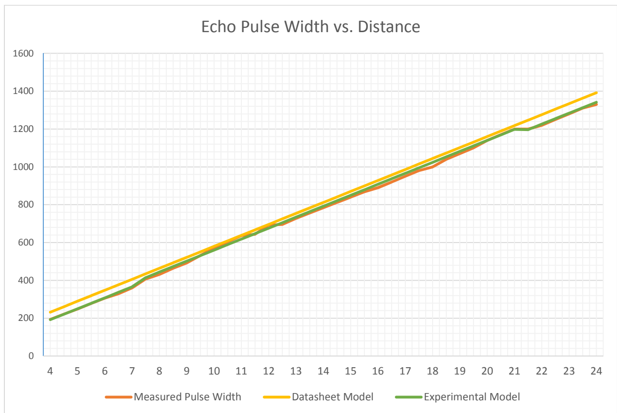
Figure E1 – Graph of Ultrasonic Sensor Test
