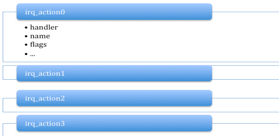
Figure 4-4: Diagram illustrating the interrupt table
