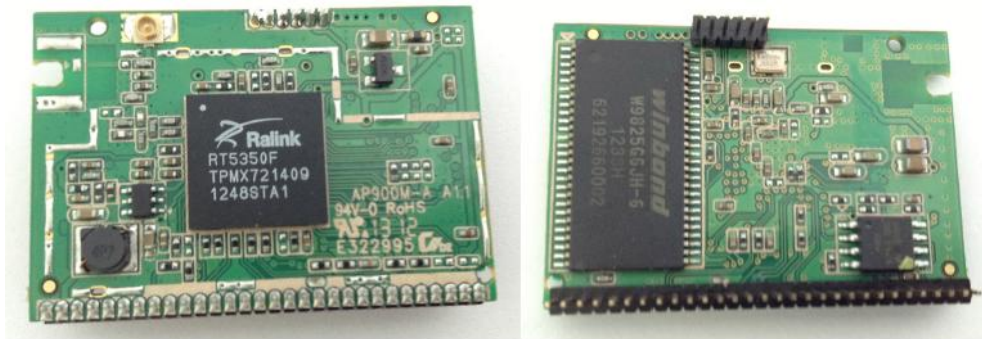
Figure 3-1: Pictures of the RT5350 SoC breakout board from third party
