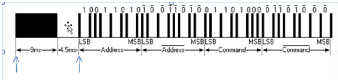
Figure 4-2: Diagram illustrating details of the NEC protocol
