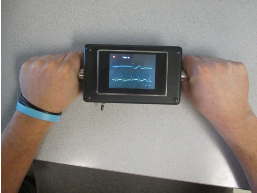
The device in action. The top line (green) has a one second time base while the bottom line (yellow) has a five second time base.
