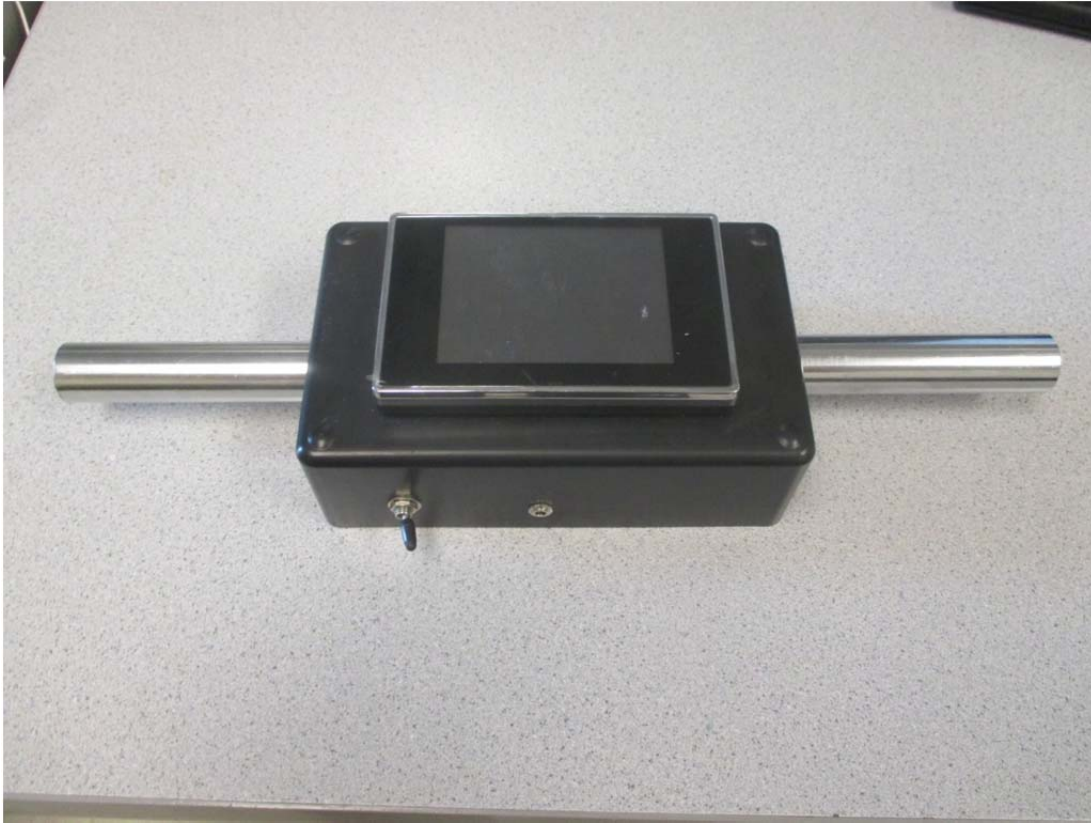
The device. The black box contains the circuit and microcontroller, the mini tv is set on top, the bars on the sides are for holding it and reading hand voltage, and the power switch is on the front along with the output jack.
