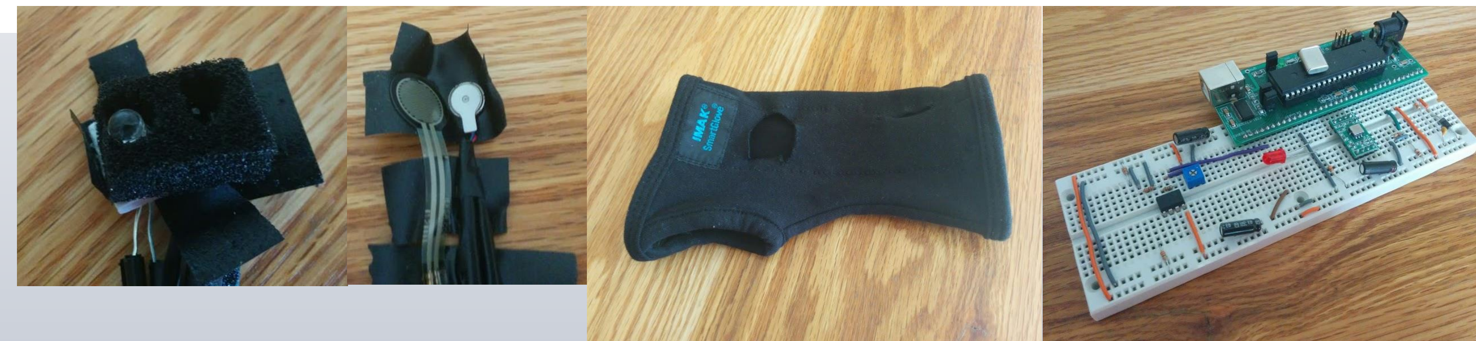
Parts Picture. (From Left to Right: IR, Pressure Sensor, Vibration Motor, Wrap, Microcontroller + Accelerometer)
